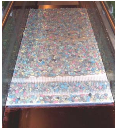
Picture 2-5: The adhesive bottom plate
