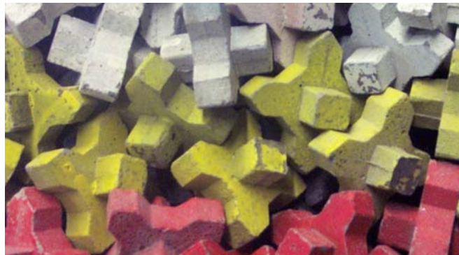
Picture 1-1: Interlocking between Xblobs (scale model)
