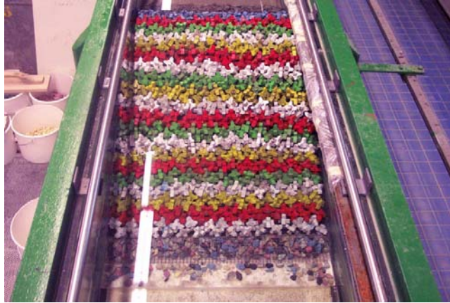
Picture 3-4: Xbloc armour after testing on mild foreshore: no damage
