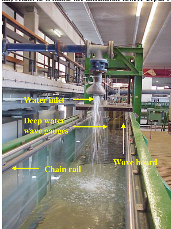
Picture 2-1: View of the wave flume, towards the wave board
