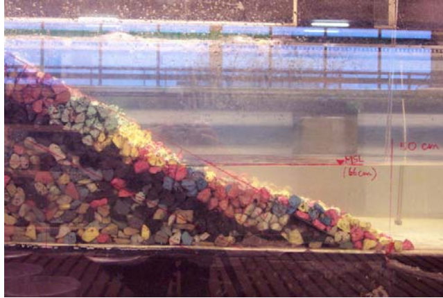
Picture 3-2: Riprap armour after testing
