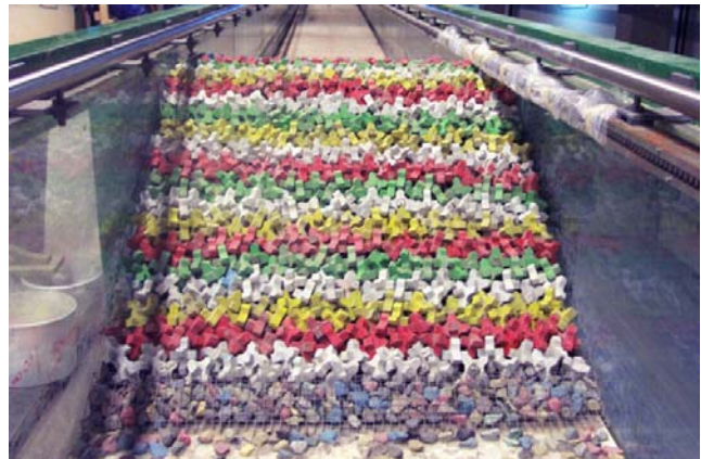
Picture 2-4: Front view of breakwater with Xbloc units
