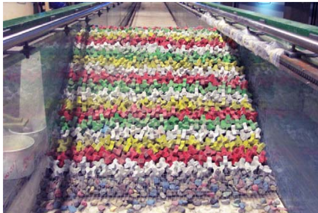
Picture 3-3: Xbloc armour layer ready for testing
