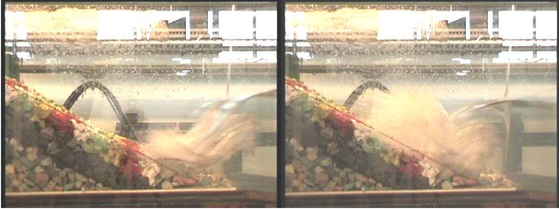
Picture 3-6: High plunging waves attacking the toe
