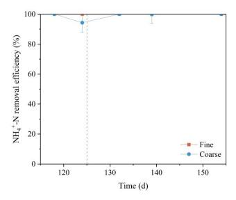
**Fig. 22.** Temporal changes in NH4+-N removal efficiency in fine and coarse columns during phase II. The dashed line indicates the start of the phase II – backwashing.
