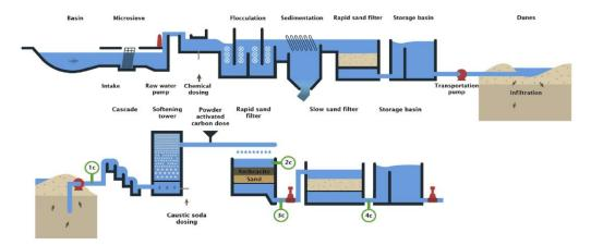
Fig. 1. Process schemes of drinking water treatment at Katwijk, the Netherlands (Ahmad et al. 2020).
