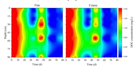
**Fig. A3.** Depth profiles of DOC in fine and coarse columns operating at 0.5 m/h during immature stage in phase I. The DOC measurements were normalized by removing background concentrations of tap water.
