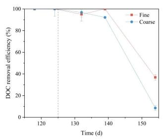
**Fig. 14.** Temporal changes in DOC removal efficiency in fine and coarse columns during phase II. The dashed line indicates the start of the phase II – increasing loading rate.
