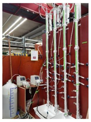
Fig. 2. Experimental set-up of lab-scale slow sand filters.
