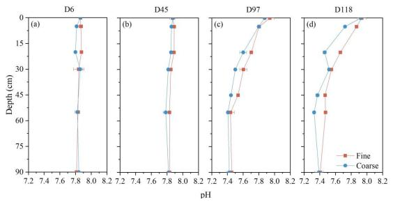
Fig. 5. Depth profile of pH within the SSFs on day 6 (a), 45 (b), 97(c), and 118 (d).
