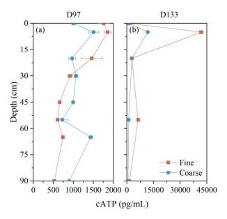
**Fig. 18.** Depth profile of cATP concentration in water before (a) and 8 days (b) after increasing loading rate.
