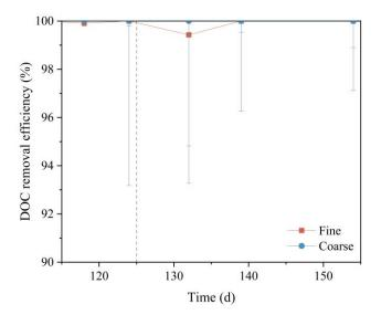
**Fig. 20.** Temporal changes in DOC removal efficiency in fine and coarse columns during phase II. The dashed line indicates the start of the phase II – backwashing.
