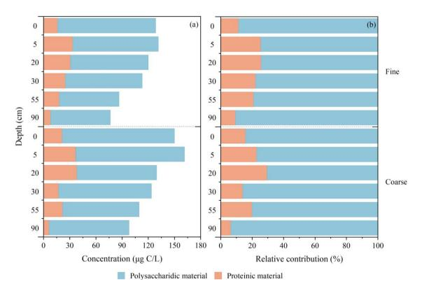
**Fig. A12.** Vertical concentrations (a) and relative distributions (b) of the polysaccharides and proteins fractions in biopolymers within the SSFs on day 106.
