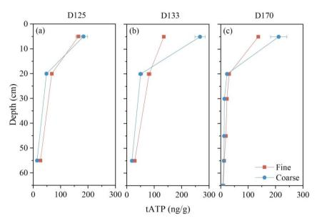
**Fig. 25.** Depth profile of deposit tATP concentration normalized to the mass of sand before backwashing (a), 8 days (b), and 45 days (c) after backwashing.
