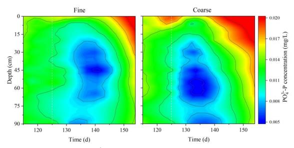
**Fig. A20.** Depth profiles of PO<sub>4</sub><sup>3</sup>-P in fine and coarse columns operating at 2 m/h during phase II. The PO<sub>4</sub><sup>3</sup>-P measurements were normalized by removing background concentrations of tap water. The dashed line indicates the start of the phase II – increasing loading rate.
