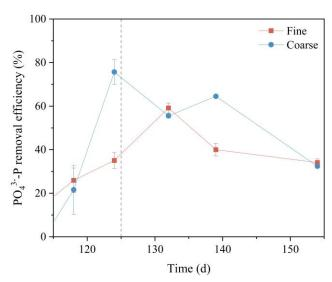
**Fig. A22.** Temporal changes in PO<sub>4</sub><sup>3</sup>--P removal efficiency in fine and coarse columns during phase II. The dashed line indicates the start of the phase II – backwashing.
