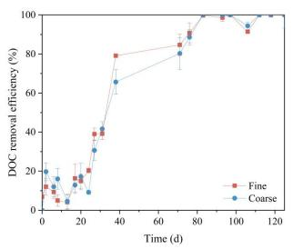
Fig. 6. Temporal changes in DOC removal efficiency in fine and coarse columns during phase I.
