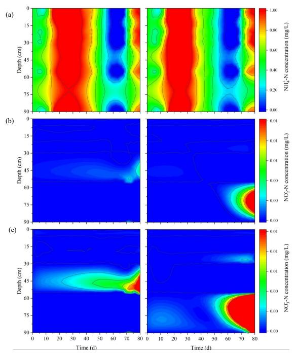
**Fig. A5.** Depth profiles of NH<sub>4</sub><sup>+</sup>-N (a), NO<sub>2</sub><sup>-</sup>-N (b), and NO<sub>3</sub><sup>-</sup>-N (c) in fine and coarse columns operating at 0.5 m/h during immature stage in phase I. The DOC measurements were normalized by removing background concentrations of tap water.
