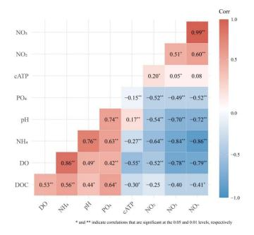
**Fig. A24.** Average correlation between physicochemical and biological parameters of filtrate water at various depths within both fine and coarse SSFs during phase I. \* and \*\* indicate differences are significant at the 0.05 and 0.01 levels, respectively.
