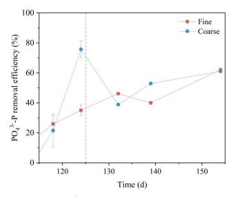
Fig. A19. Temporal changes in  $PO_4^{3-}$ -P removal efficiency in fine and coarse columns during phase II. The dashed line indicates the start of the phase II – increasing loading rate.
