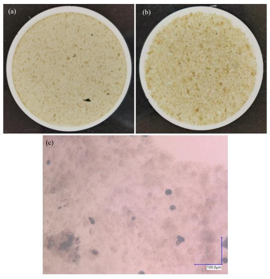
**Fig. A18.** Photos of the flocs in the wastewater of hydraulic washing from fine (a) and coarse (b) columns on 0.45 um on day 152. And the electron microscope image of floc (c).
