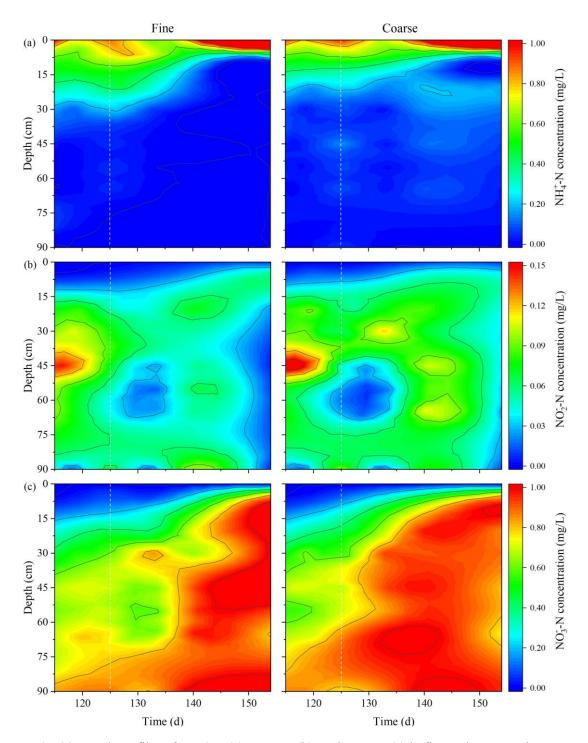
**Fig. 23.** Depth profiles of NH<sub>4</sub><sup>+</sup>-N (a), NO<sub>2</sub><sup>-</sup>-N (b), and NO<sub>3</sub><sup>-</sup>-N (c) in fine and coarse columns operating at 0.5 m/h during phase II. The measurements were normalized by removing background concentrations of tap water. The dashed line indicates the start of phase II - backwashing.
