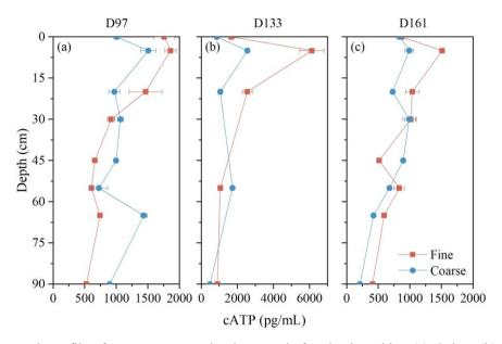
**Fig. 24.** Depth profile of cATP concentration in water before backwashing (a), 8 days (b), and 36 days (c) after backwashing.
