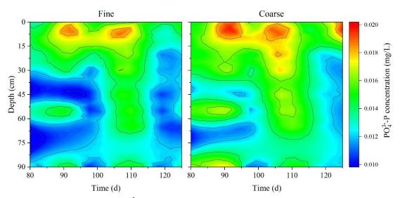
**Fig. A16.** Depth profiles of PO<sub>4</sub><sup>3</sup>-P in fine and coarse columns operating at 0.5 m/h in phase I. The PO<sub>4</sub><sup>3</sup>-P measurements were normalized by removing background concentrations of tap water.
