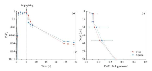
Fig. A7. Breakthrough curve (a) and log removal over the height (b) of PhiX 174 in SSFs.
