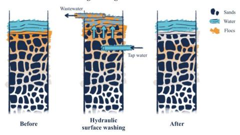
Fig. A17. Schemes of hydraulic surface cleaning.
