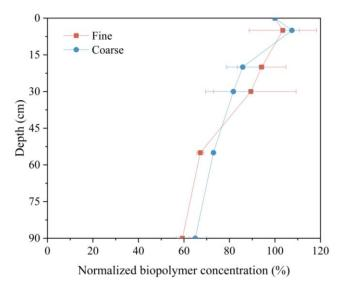
Fig. A11. Biopolymer removal profile in fine and coarse columns on day 106.
