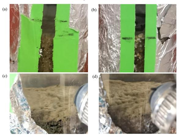
**Fig. A21.** Photos of the surface of fine and coarse filter columns before (a, b) and after (c, d) backwashing.
