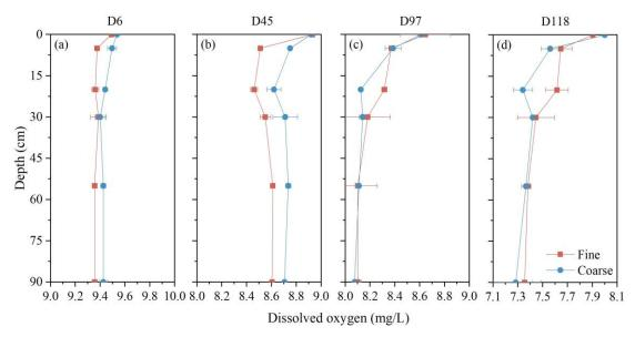
Fig. 4. Depth profile of DO concentration within the SSFs on day 6 (a), 45 (b), 97(c), and 118 (d).
