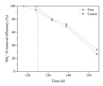
**Fig. 16.** Temporal changes in NH<sub>4</sub><sup>+</sup>-N removal efficiency in fine and coarse columns during phase II. The dashed line indicates the start of the phase II – increasing loading rate.
