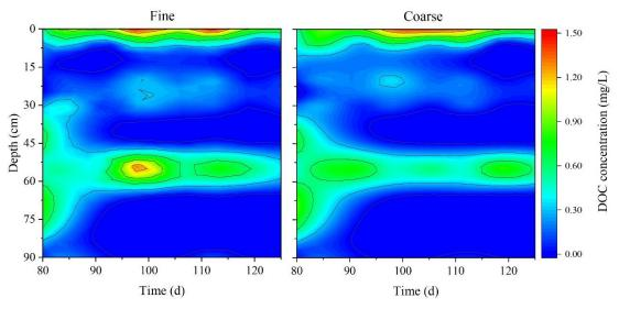
**Fig. 7.** Depth profiles of DOC in fine and coarse columns operating at 0.5 m/h. The DOC measurements were normalized by removing background concentrations of tap water.
