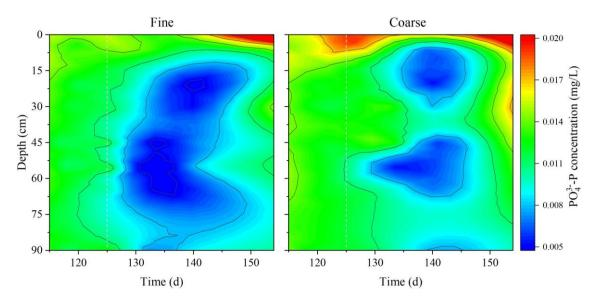
**Fig. A23.** Depth profiles of PO<sub>4</sub><sup>3-</sup>-P in fine and coarse columns operating at 0.5 m/h during phase II. The PO<sub>4</sub><sup>3-</sup>-P measurements were normalized by removing background concentrations of tap water. The dashed line indicates the start of the phase II – backwashing.
