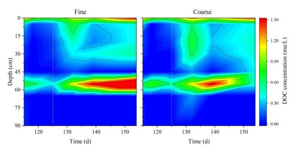
**Fig. 21.** Depth profiles of DOC in fine and coarse columns operating at 0.5 m/h during phase II. The DOC measurements were normalized by removing background concentrations of tap water.
