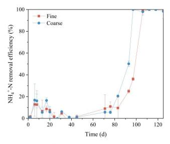
Fig. 10. Temporal changes in NH<sub>4</sub><sup>+</sup>-N removal efficiency in fine and coarse columns during phase I.
