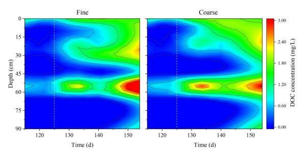
**Fig. 15.** Depth profiles of DOC in fine and coarse columns operating at 2 m/h during phase II. The DOC measurements were normalized by removing background concentrations of tap water. The dashed line indicates the start of the phase II – increasing loading rate.
