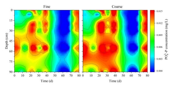
**Fig. A4.** Depth profiles of PO<sub>4</sub><sup>3</sup>-P in fine and coarse columns operating at 0.5 m/h during immature stage in phase I. The DOC measurements were normalized by removing background concentrations of tap water.
