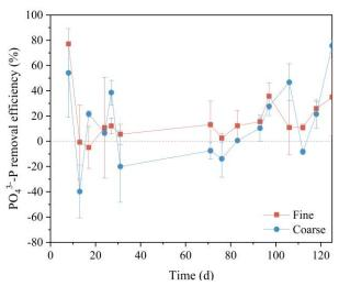
Fig. A15. Temporal changes in PO<sub>4</sub><sup>3</sup>-P removal efficiency in fine and coarse columns during phase I.
