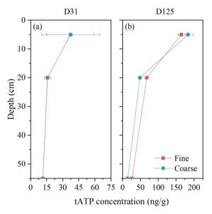
**Fig. 13.** Depth profile of deposit tATP concentration normalized to the mass of sand on day 31(a) and 125 (b).
