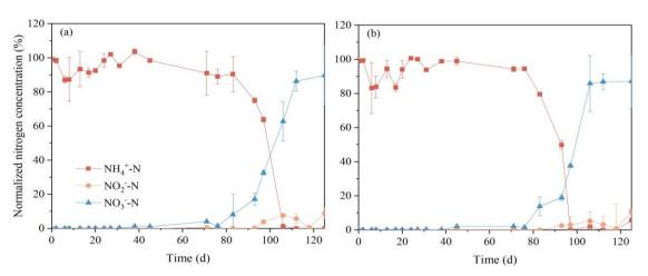
**Fig. 9.** Nitrogen conversion profile between NH<sub>4</sub><sup>+</sup>-N, NO<sub>2</sub><sup>-</sup>-N, and NO<sub>3</sub><sup>-</sup>-N within fine (a) and coarse (b) columns during the phase I. The concentrations are normalized by dividing the influent NH<sub>4</sub><sup>+</sup>-N.
