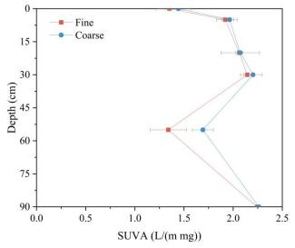
Fig. A13. Depth profile of SUVA in fine and coarse columns on day 106.
