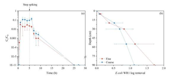
Fig. A6. Breakthrough curve (a) and log removal over the height (b) of *E.coli* WR1 in SSFs.
