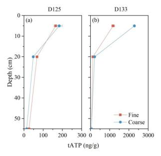
**Fig. 19.** Depth profile of deposit tATP concentration normalized to the mass of sand before (a) and 8 days (b) after increasing loading rate.
