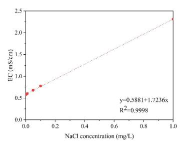
Fig. A1. Calibration curve of NaCl concentration and electric conductivity in tap water at 15 °C.
