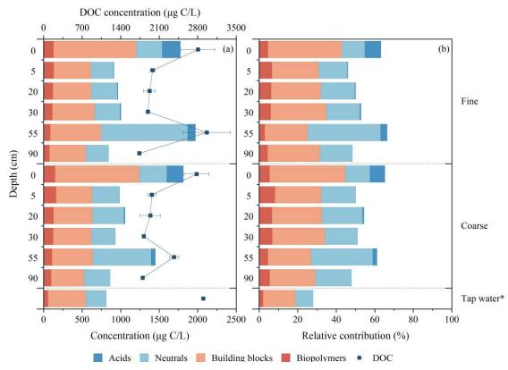
**Fig. 8.** Vertical concentrations (a) and relative distributions (b) of the DOC fractions within the SSFs on day 106. \* The data for tap water referred to (Baghoth et al. 2008).
