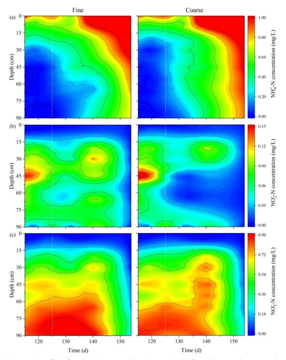
**Fig. 17.** Depth profiles of NH<sub>4</sub><sup>+</sup>-N (a), NO<sub>2</sub><sup>-</sup>-N (b), and NO<sub>3</sub><sup>-</sup>-N (c) in fine and coarse columns operating at 2 m/h during phase II. The measurements were normalized by removing background concentrations of tap water. The dashed line indicates the start of the phase II – increasing loading rate.
