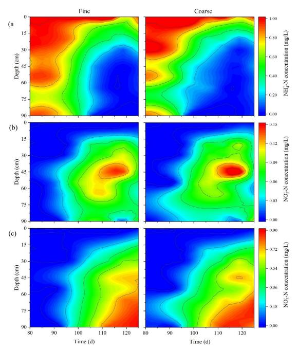
**Fig. 11.** Depth profiles of NH<sub>4</sub><sup>+</sup>-N (a), NO<sub>2</sub><sup>-</sup>-N (b), and NO<sub>3</sub><sup>-</sup>-N (c) in fine and coarse columns operating at 0.5 m/h during phase I. The measurements were normalized by removing background concentrations of tap water.
