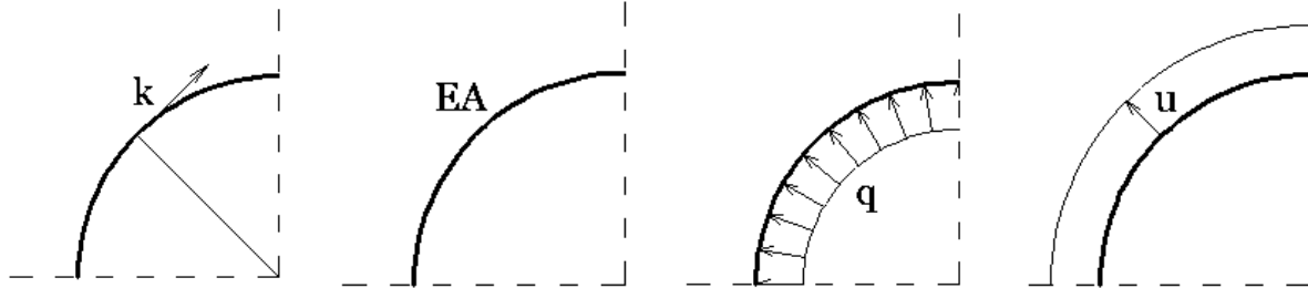
Figure 2.30 Key factors that influence the ring action in a spoke wheel roof: curvature, extensional rigidity, loads and translation
