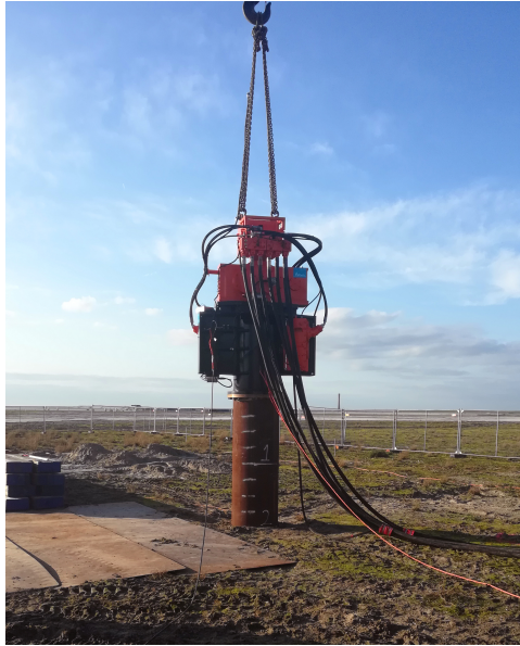
Figure 6.1: Photograph of the GDP shaker on top of a driven monopile during the GDP experimental campaign.
