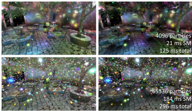
Figure 17: Examples of glowing-particle rendering without (left) and with (right) shadows. By simply setting the view volume to a sphere, we can render shadow maps for glowing particles.
