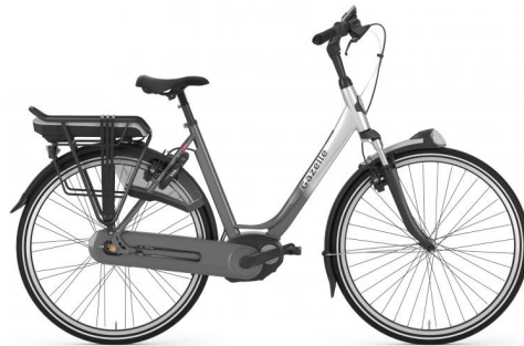
Figure 8: Orange HMB, with a crank motor
