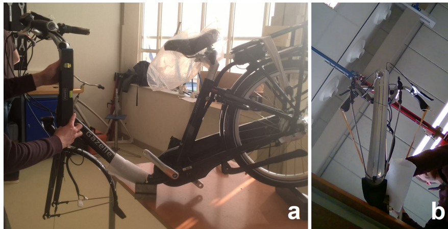
Figure 43: a. Position of the bicycle with a vertical head tube. b. Test-setup with elastics from camera view
