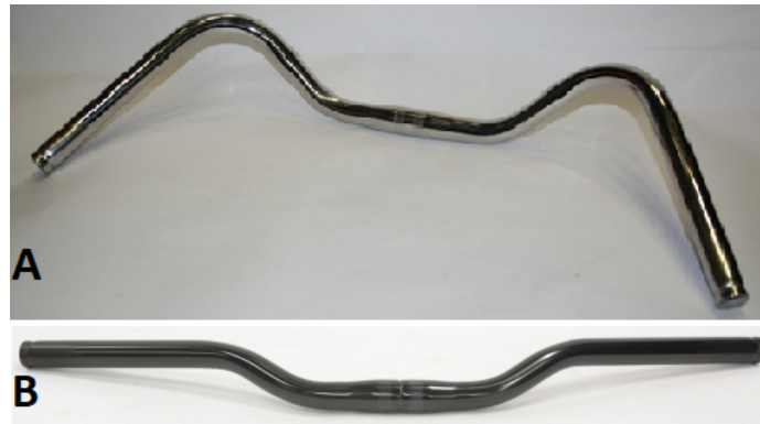
Figure 2: A. Steer with a large angle in the handlebars[8]. B. Steer with a small angle in the handlebars[9]
