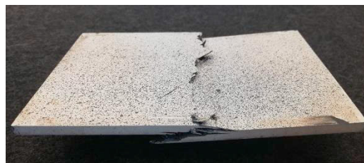
Fig. 4. Failed fatigue specimen showing the presence of delamination and kinking in transverse direction
