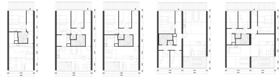
FIG. 57 Representation of various room configurations and room dimensions [however not combined] derived from the typological study
