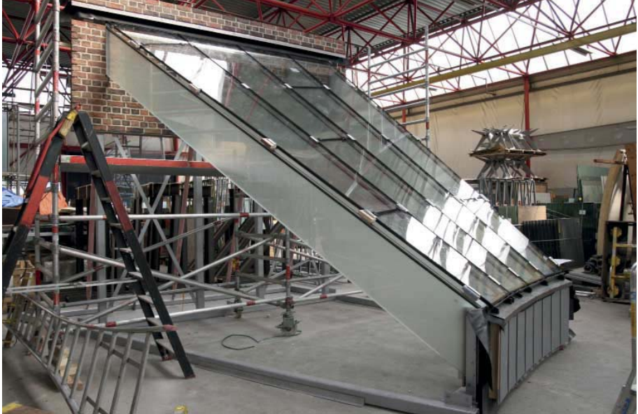
FIG. 04 Prototype with glass fins and cold twisted double glazed panels for the glass roof of the Victoria & Albert Museum London, in the Octatube laboratory
