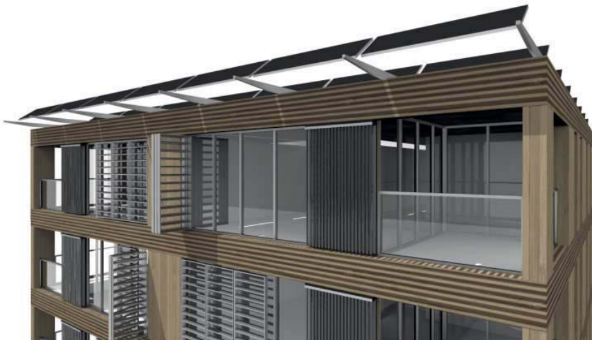
FIG. 45 Study of elements of preservation in the concept house 'Delft' prototype, and the method of integration (sun shading and heat collectors in facades) and maximisation (surface area PV on flat roof).
