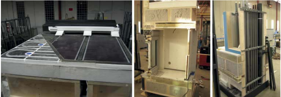
FIG. 14 Intermediate mock-ups of the essential construction nodes at true scale. [Bouweurs February 2011]
