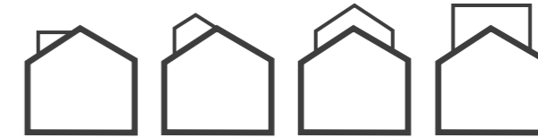
figure 33: typologies of roof structures, from left to right: roof dormer - extended roof dormer - roof structure elevated cam - roof structure elevated cam flat roof (source: own image)
