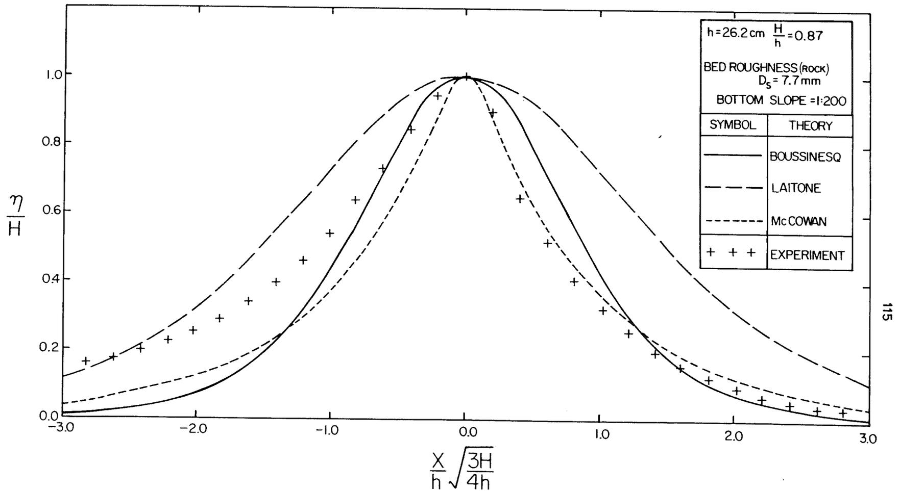
Fig. 5.6 Comparison between a measured solitary wave and between the theories of Boussinesq, McCowan, and Laitone;  $h=26.2 \text{ cm}$ ;  $H/h=0.87$ ; bottom slope=1:200.
