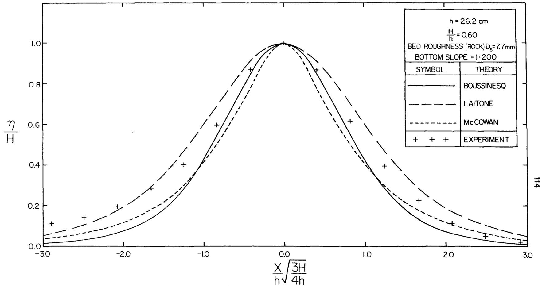
Fig. 5.5 Comparison between a measured solitary wave and between the theories of Boussinesq, McCowan, and Laitone;  $h=26.2 \text{ cm}$ ;  $H/h=0.60$ ; bottom slope=1:200.
