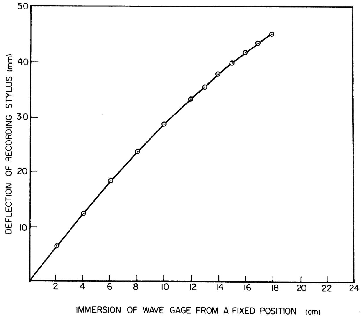
Fig. 4.7 Typical calibration curve for a wave gage.
