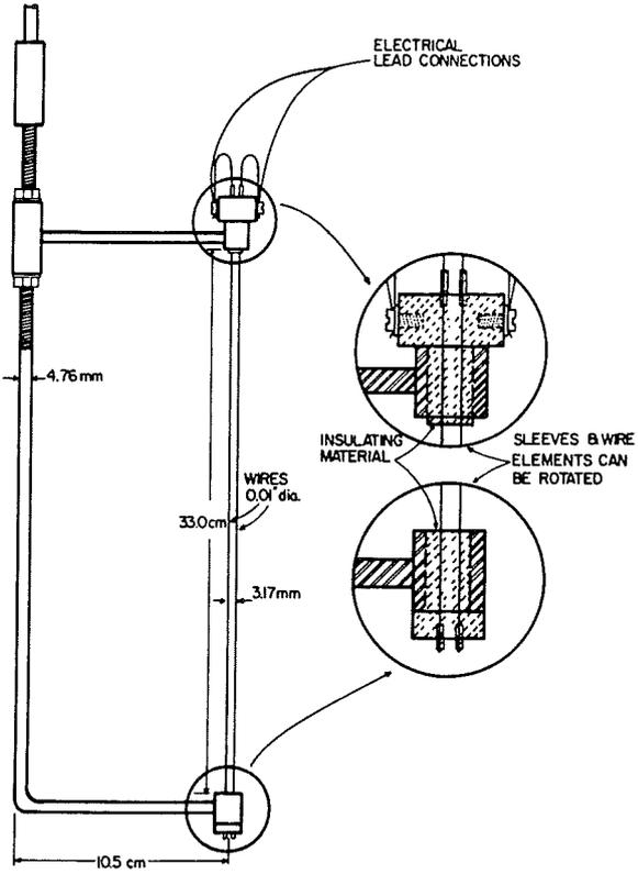
Fig. 4.5 Drawing of a typical wave gage.
