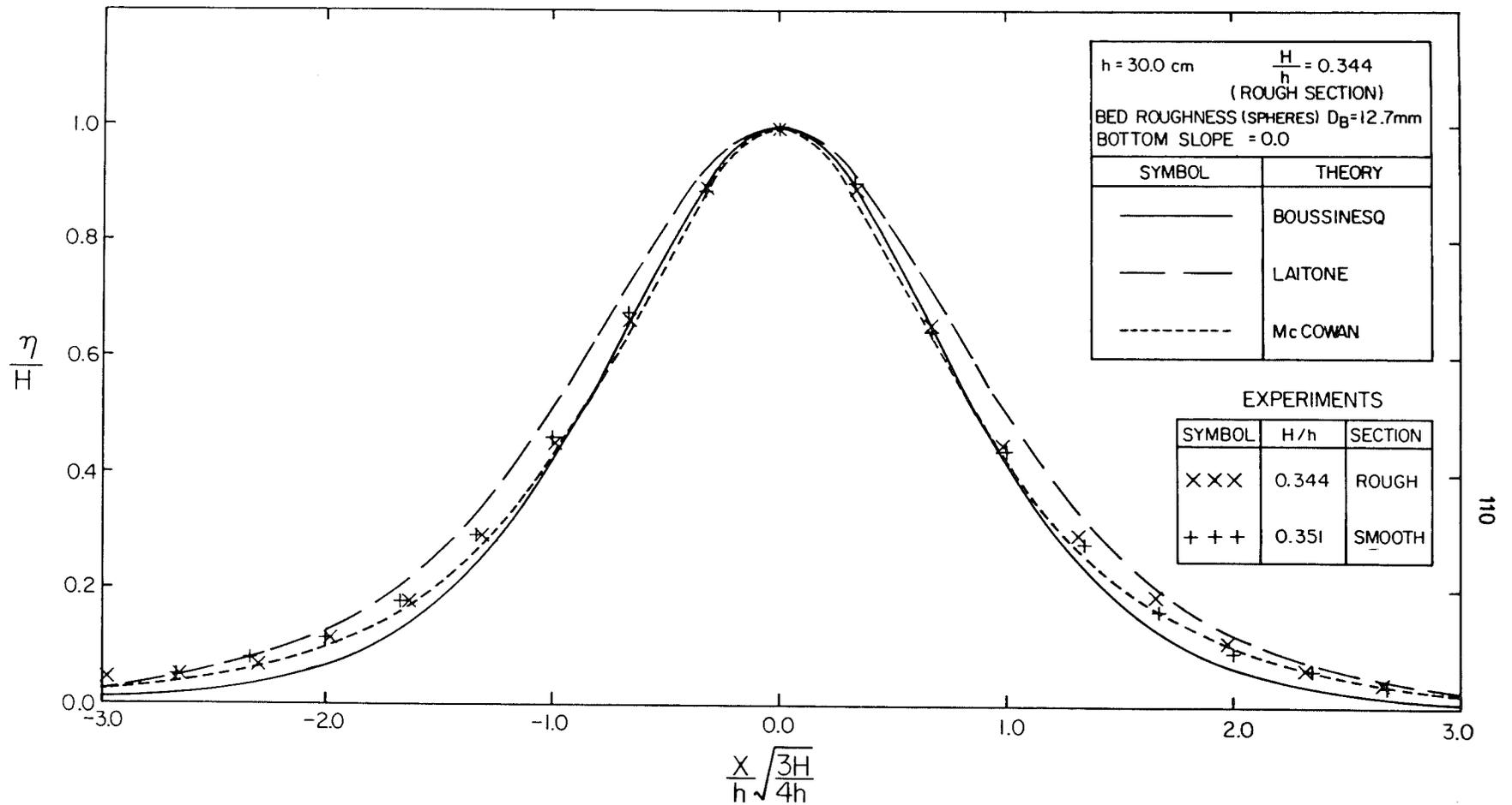
Fig. 5.2 Comparison between the solitary waves measured over the smooth and rough bed sections and between the theories of Boussinesq, McCowan, and Laitone;  $h=30.0 \text{ cm}$ ; bottom slope=0.0;  $H/h=0.351$  (over the smooth section);  $H/h=0.344$  (over the rough section).
