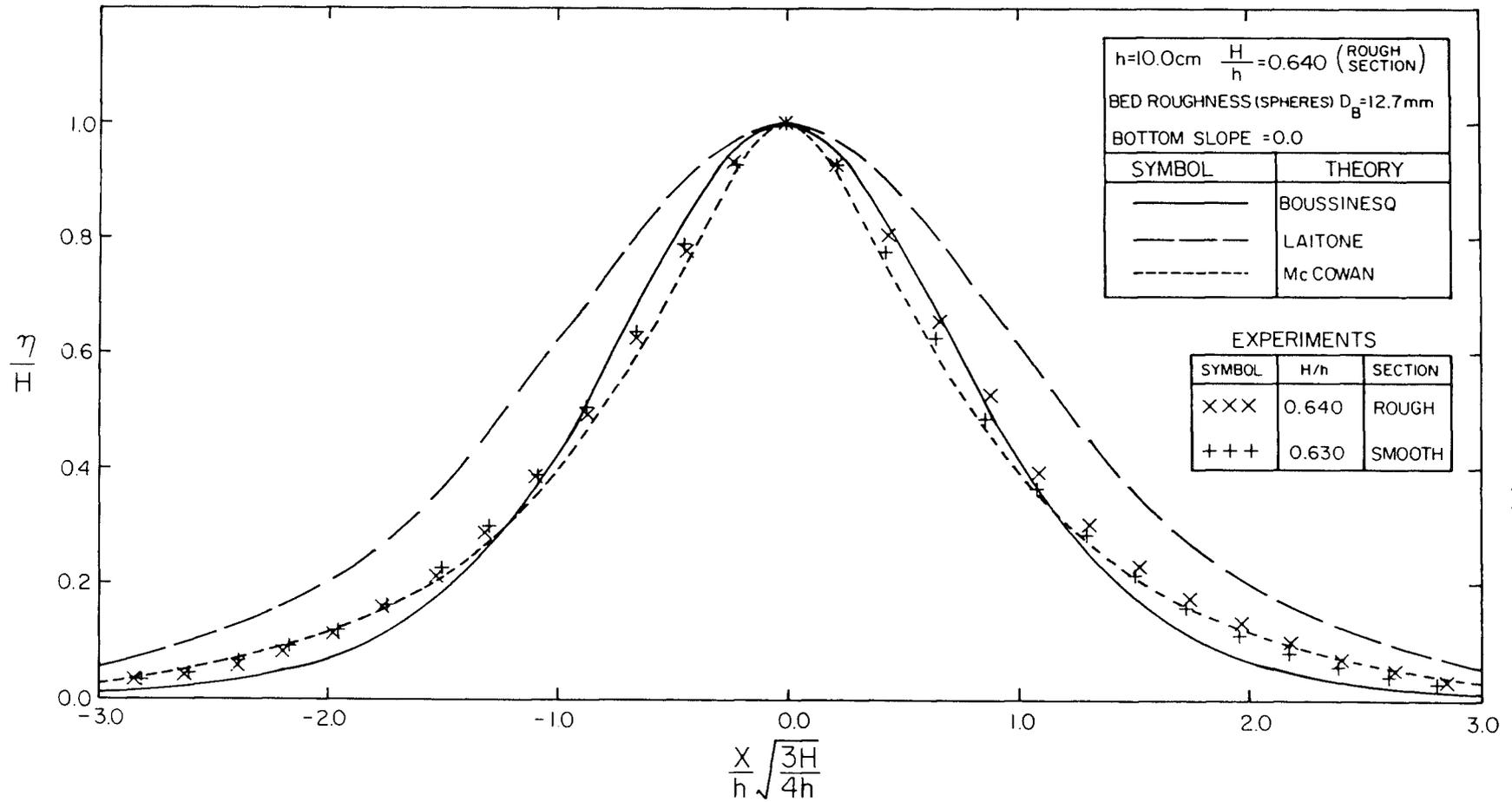
Fig. 5.3 Comparison between the solitary waves measured over the smooth and rough bed sections and between the theories of Boussinesq, McCowan, and Laitone;  $h=10.0$  cm; bottom slope=0.0;  $H/h=6.30$  (over the smooth section);  $H/h=0.640$  (over the rough section).
