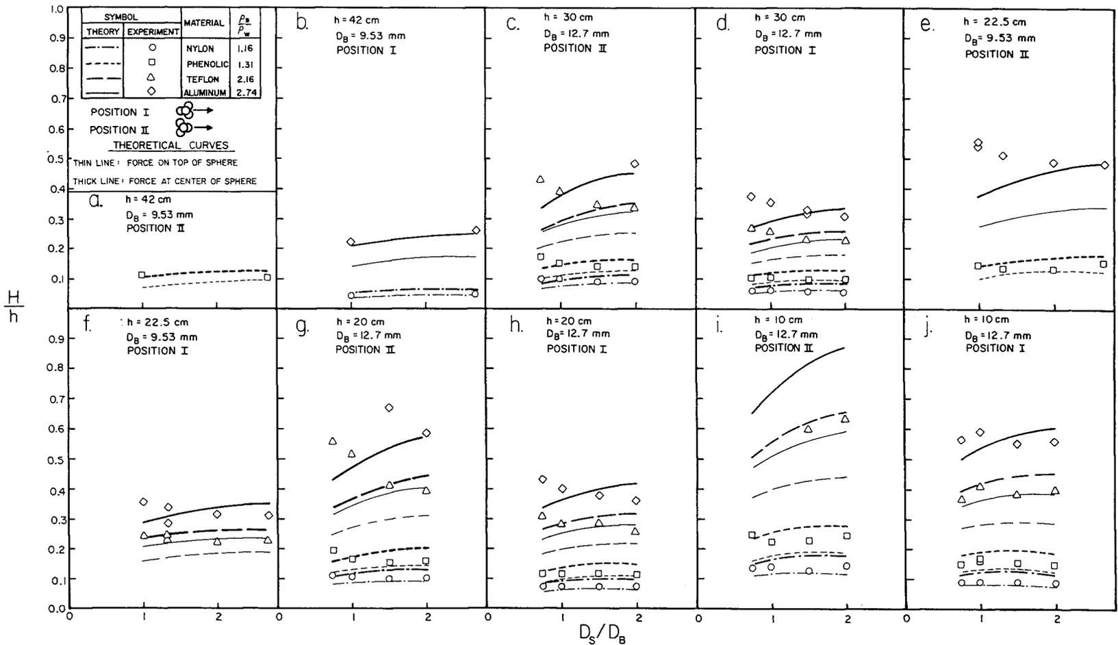
Fig. 5.24 Comparison between the experimental results of the incipient motion of spheres and the theoretical predictions (using Boussinesq's theory) assuming that the hydrodynamic forces act either at the top or at the center of the sphere.
