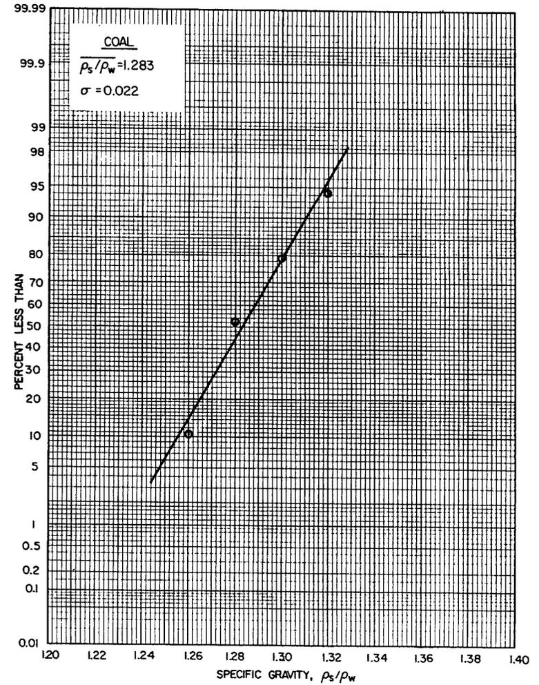
Fig. 4.20 Specific gravity distribution curves of the materials used in the experiments; (a) Natural rock, (b) Coal.
