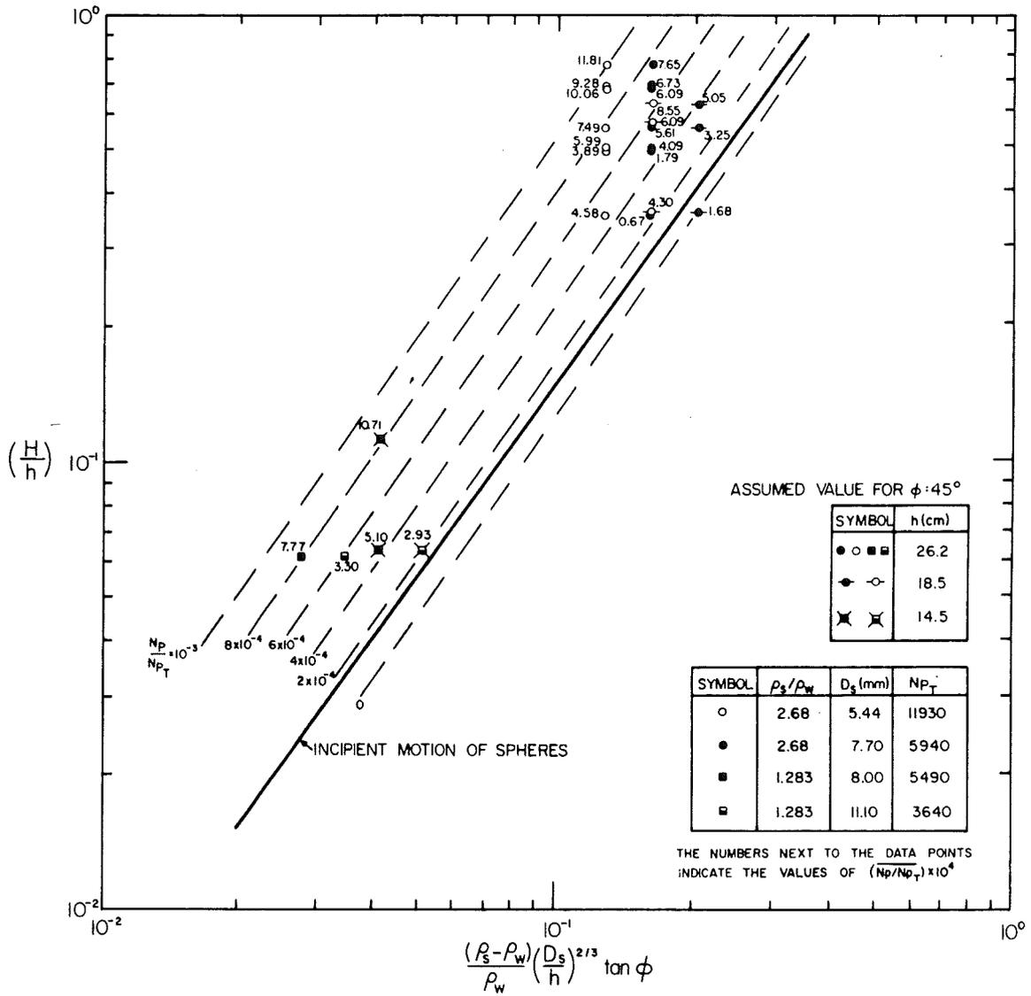
Fig. 5.30 The average amount of motion of particles of arbitrary shape as a function of the wave height, the water depth, the angle  $\phi$ , and the mean diameter and submerged density of the particles.
