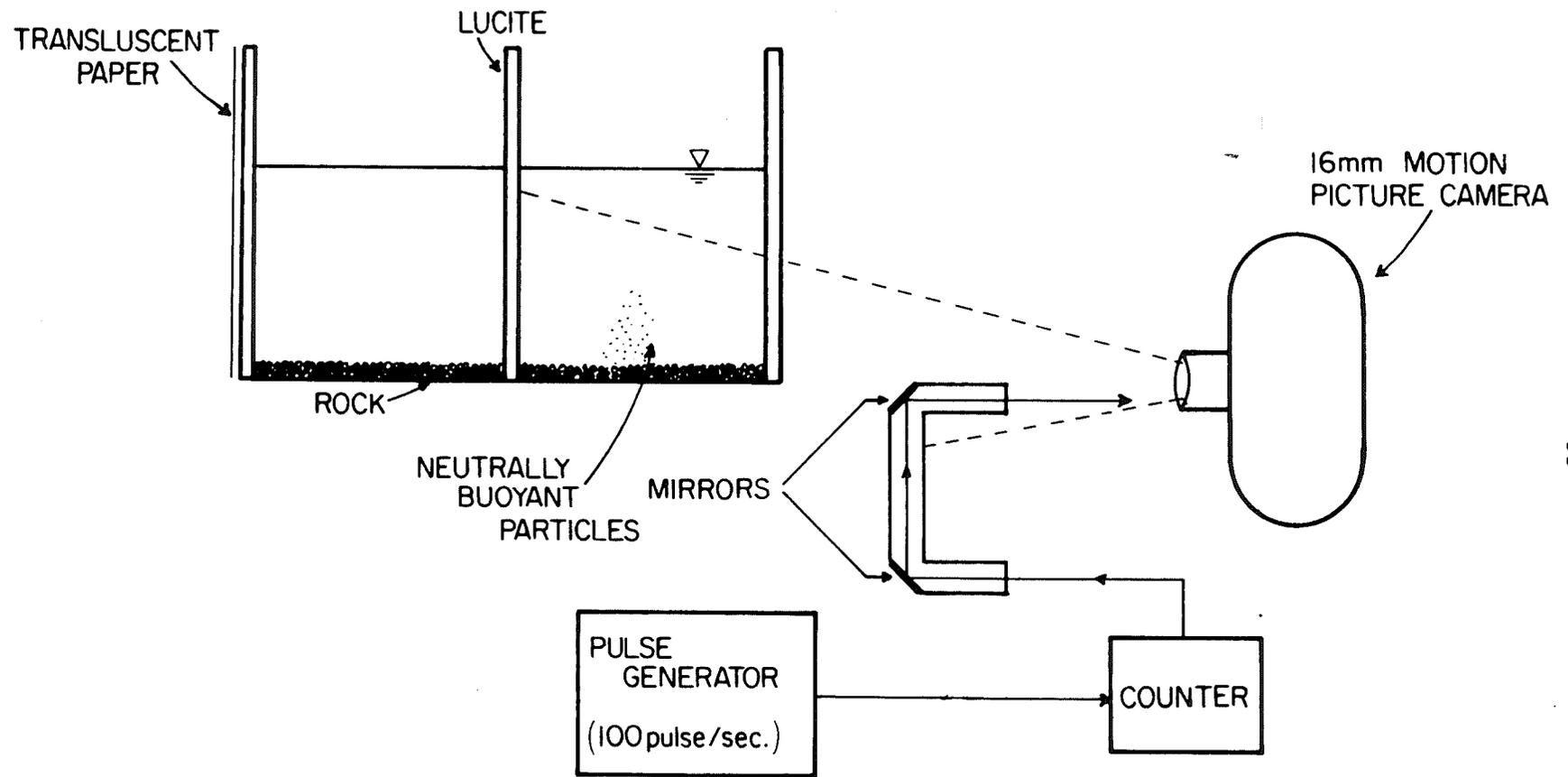
Fig. 4.27 Schematic drawing of the system used to measure the fluid particle velocity.
