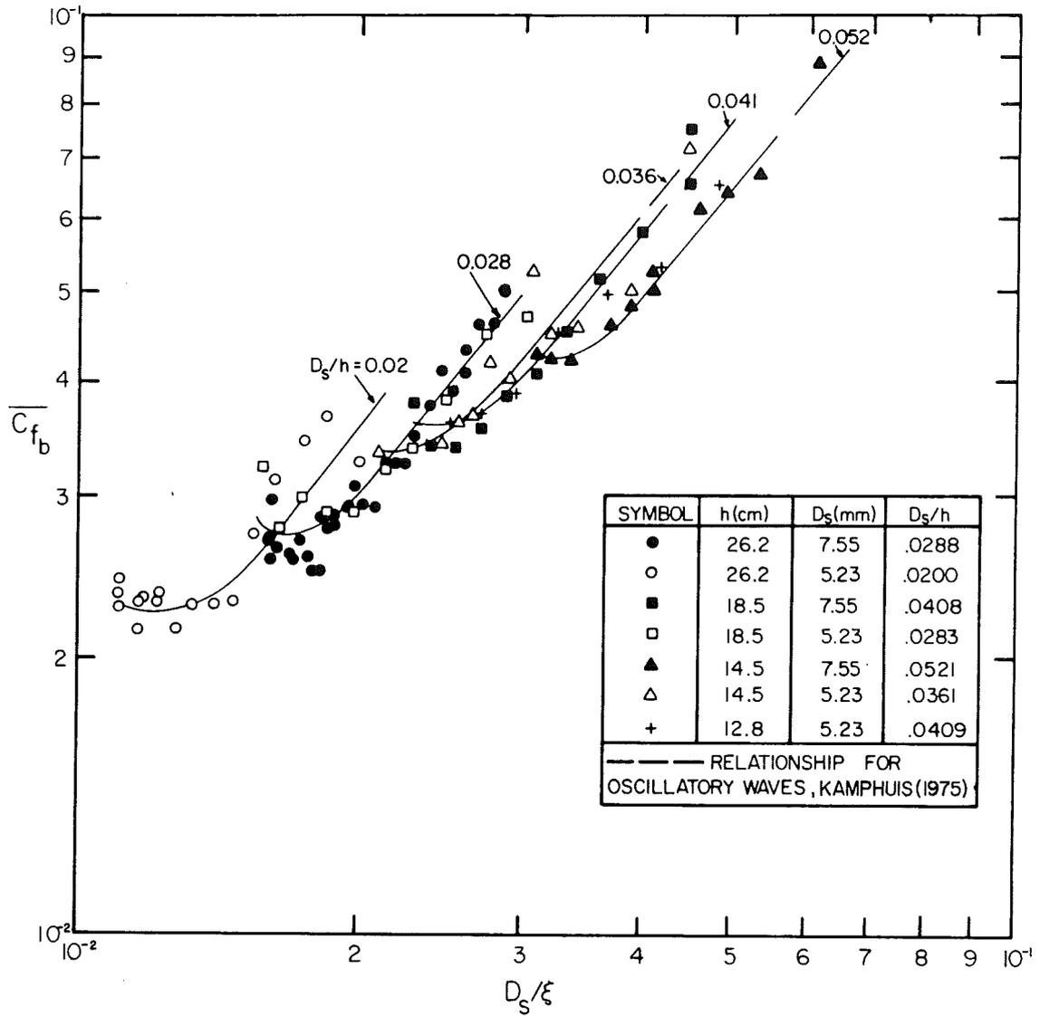
Fig. 5.12 The mean resistance coefficient as a function of the ratio of the roughness size,  $D_s$ , to the displacement of a fluid particle just outside the boundary layer,  $\xi$ .
