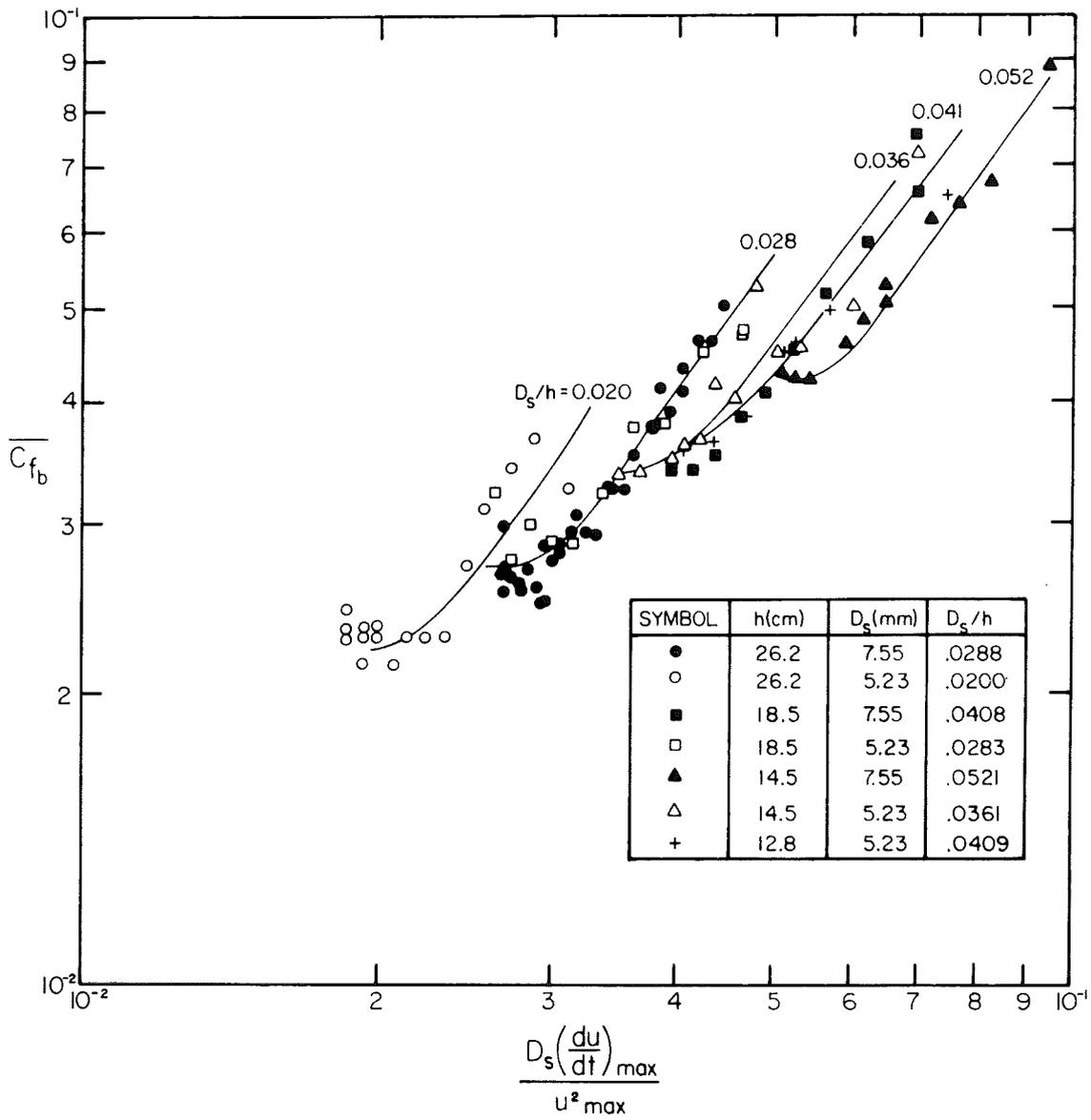
Fig. 5.13 The mean resistance coefficient as a function of the characteristic dimensionless acceleration.
