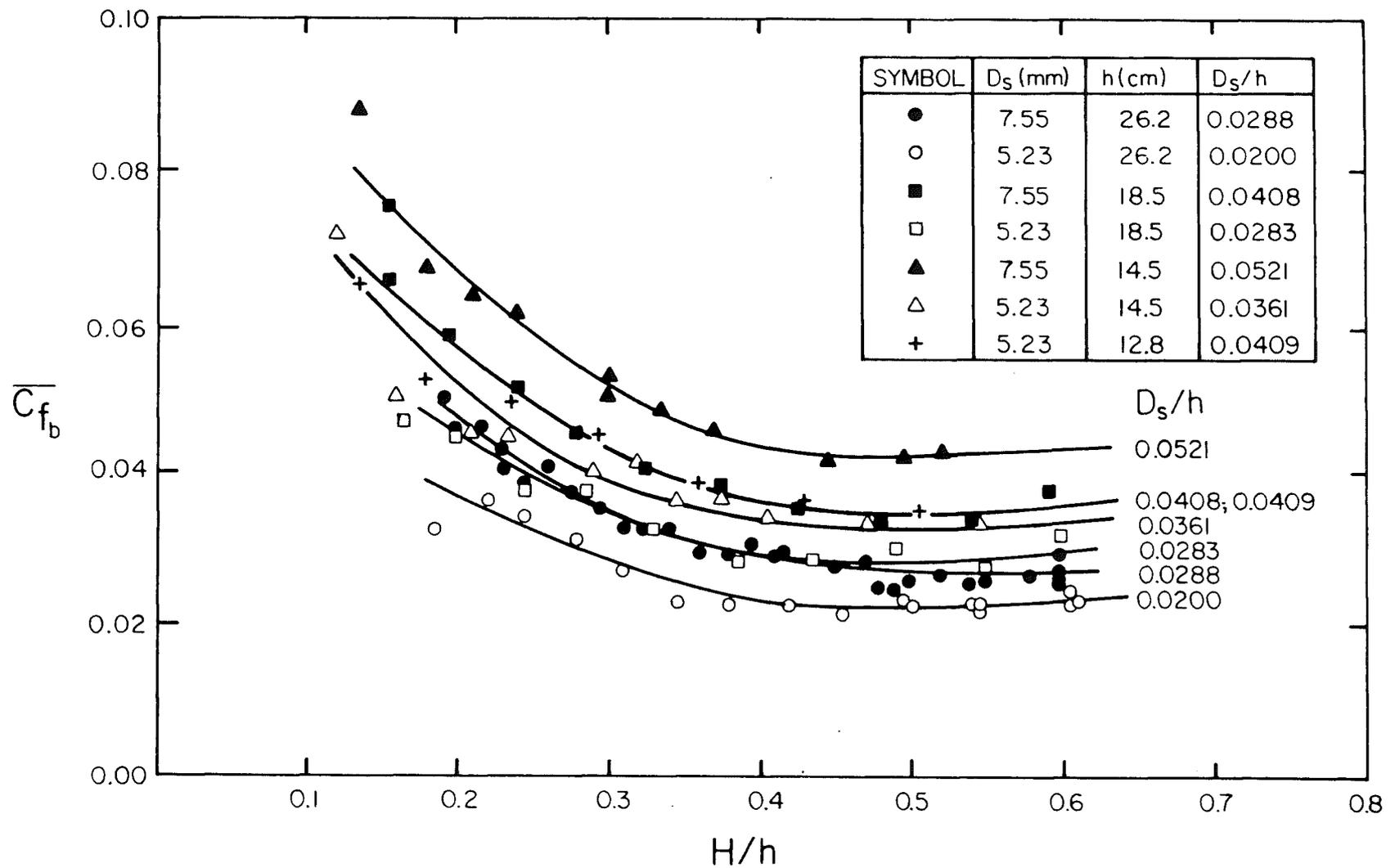
Fig. 5.14 The mean resistance coefficient as a function of the dimensionless lengths  $H/h$  and  $D_s/h$ .
