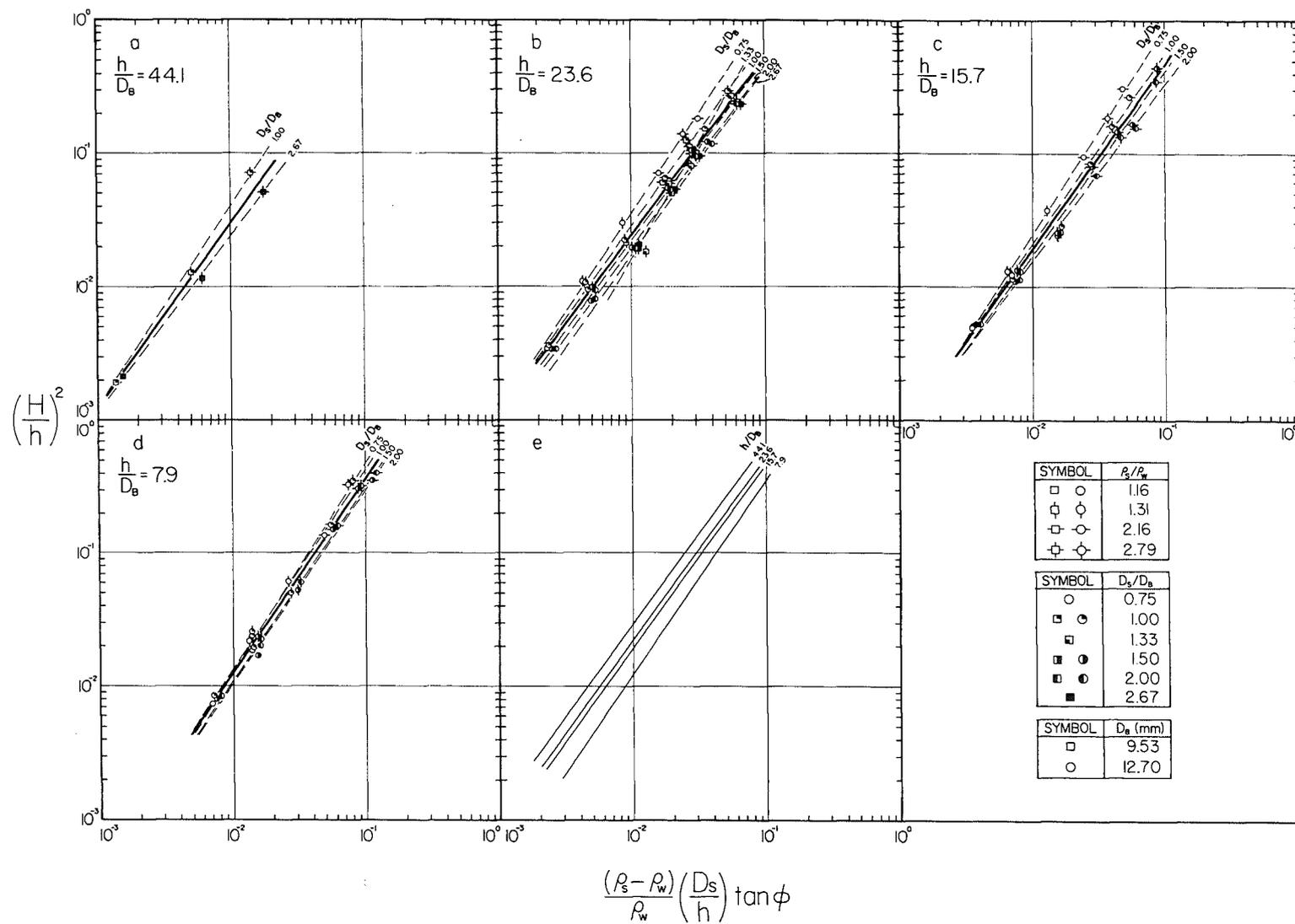
Fig. 5.25 Experimental results of the incipient motion of spheres.
