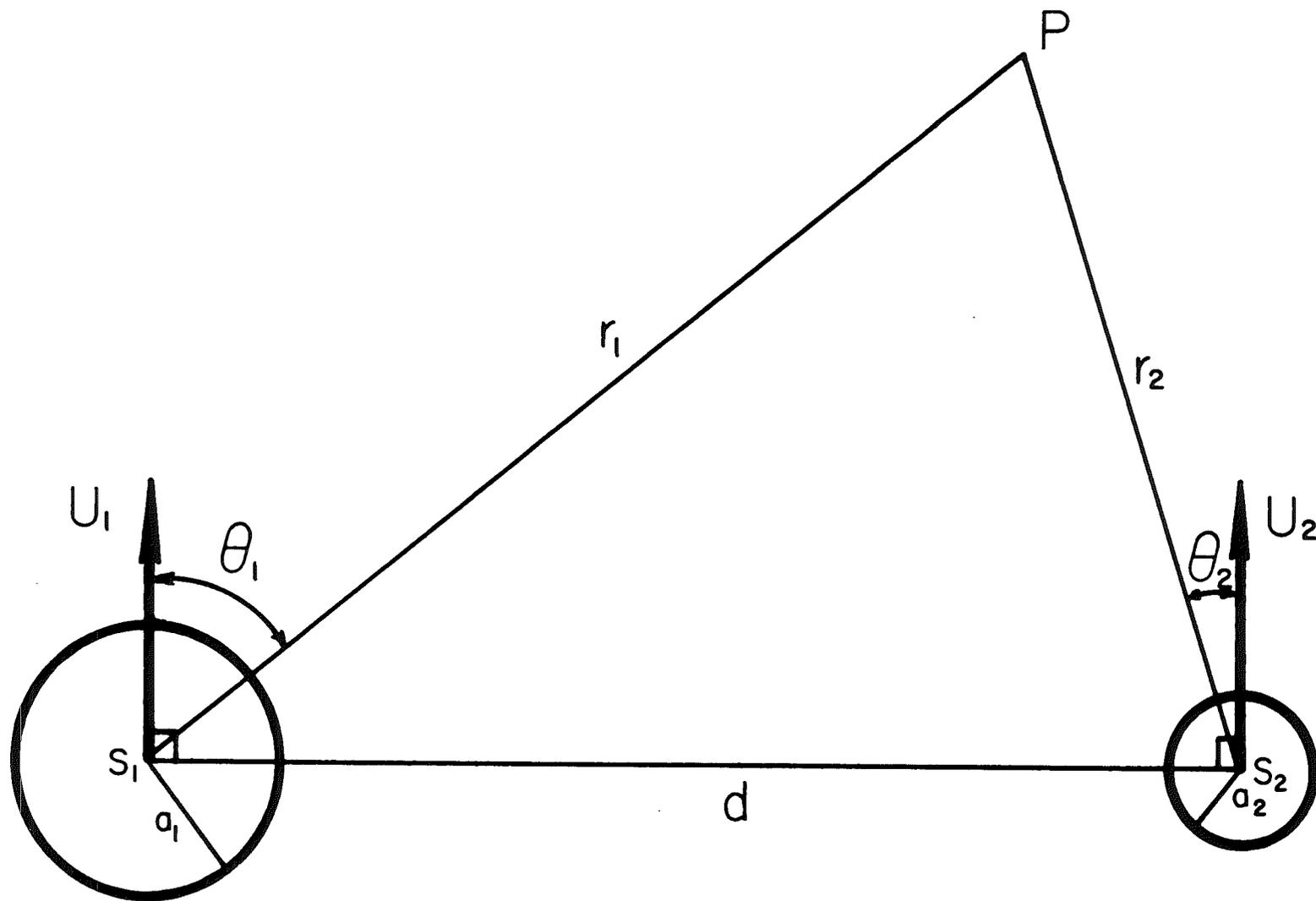
Fig. A.1.1 Definition sketch for the motion of two spheres in a fluid.
