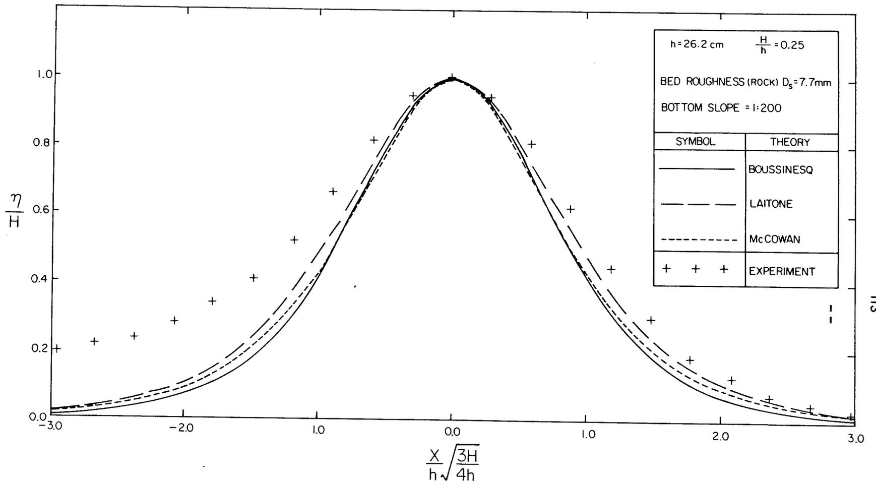
Fig. 5.4 Comparison between a measured solitary wave and between the theories of Boussinesq, McCowan, and Laitone;  $h=26.2 \text{ cm}$ ;  $H/h=0.25$ ; bottom slope=1:200.
