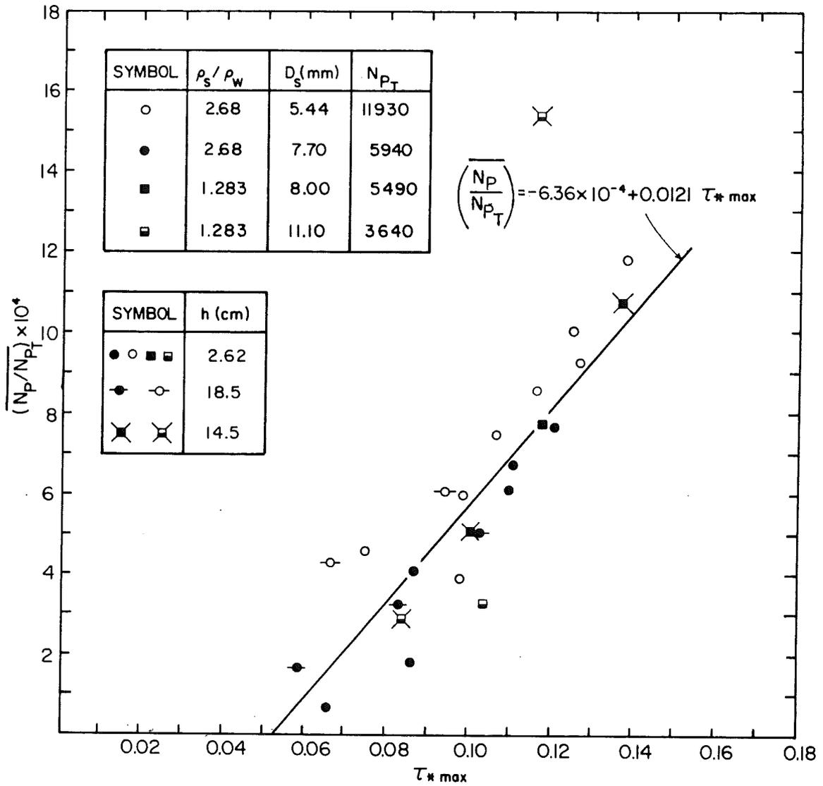
Fig. 5.18 The average amount of motion of particles of arbitrary shape as a function of the dimensionless shear stress.
