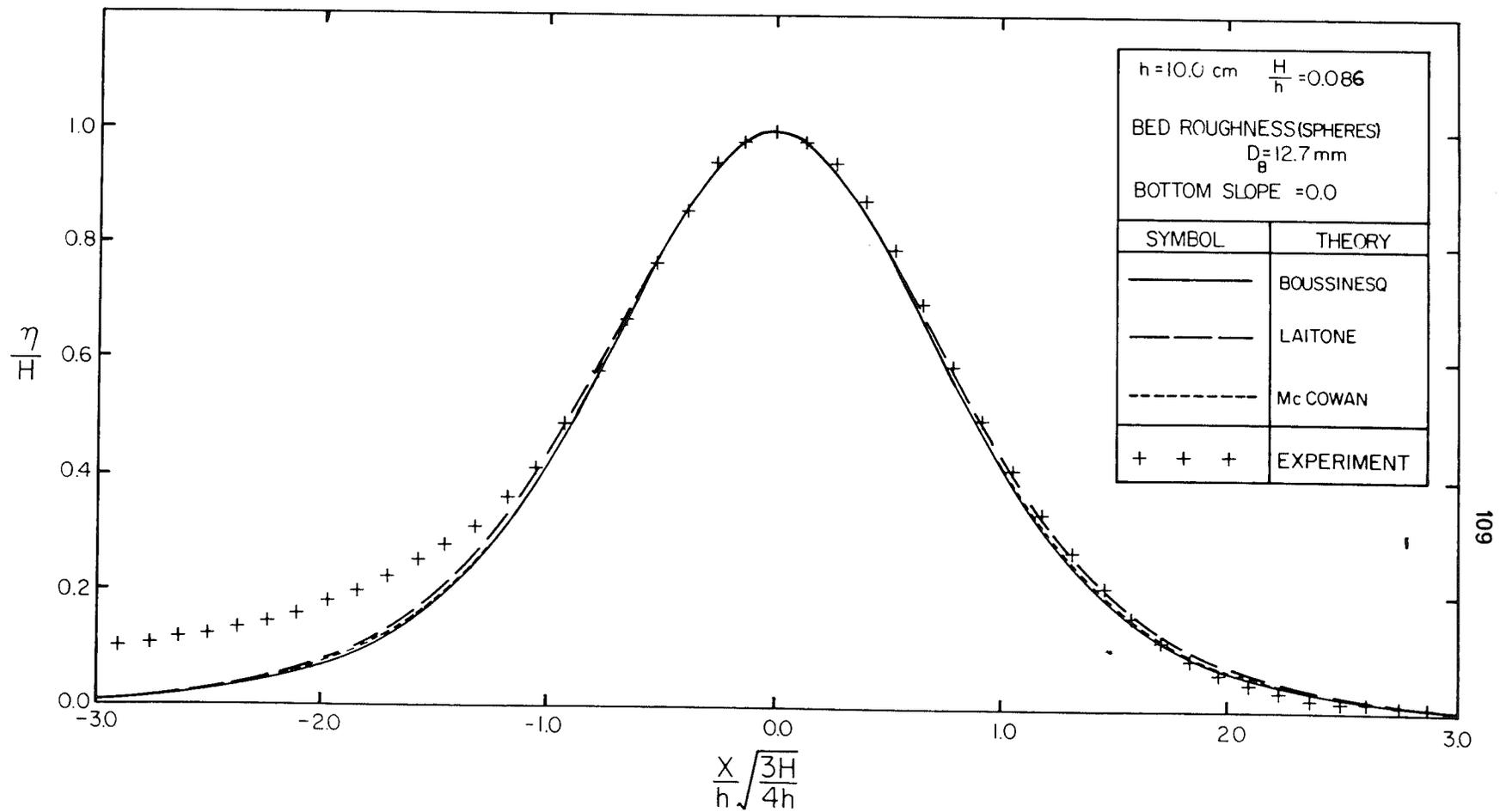
Fig. 5.1 Comparison between a measured solitary wave and between the theories of Boussinesq, McCowan, and Laitone;  $h=10.0 \text{ cm}$ ;  $H/h=0.086$ ; bottom slope=0.0.
