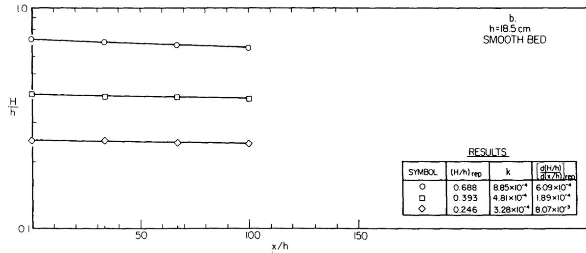
Fig. 5.10 Attenuation of solitary waves along a channel; (a) over a rough bed; (b) over a smooth bed.
