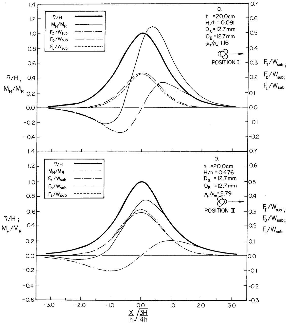
Fig. 5.22 The distribution of forces and moments exerted on a sphere under solitary waves (using McCowan's theory).
