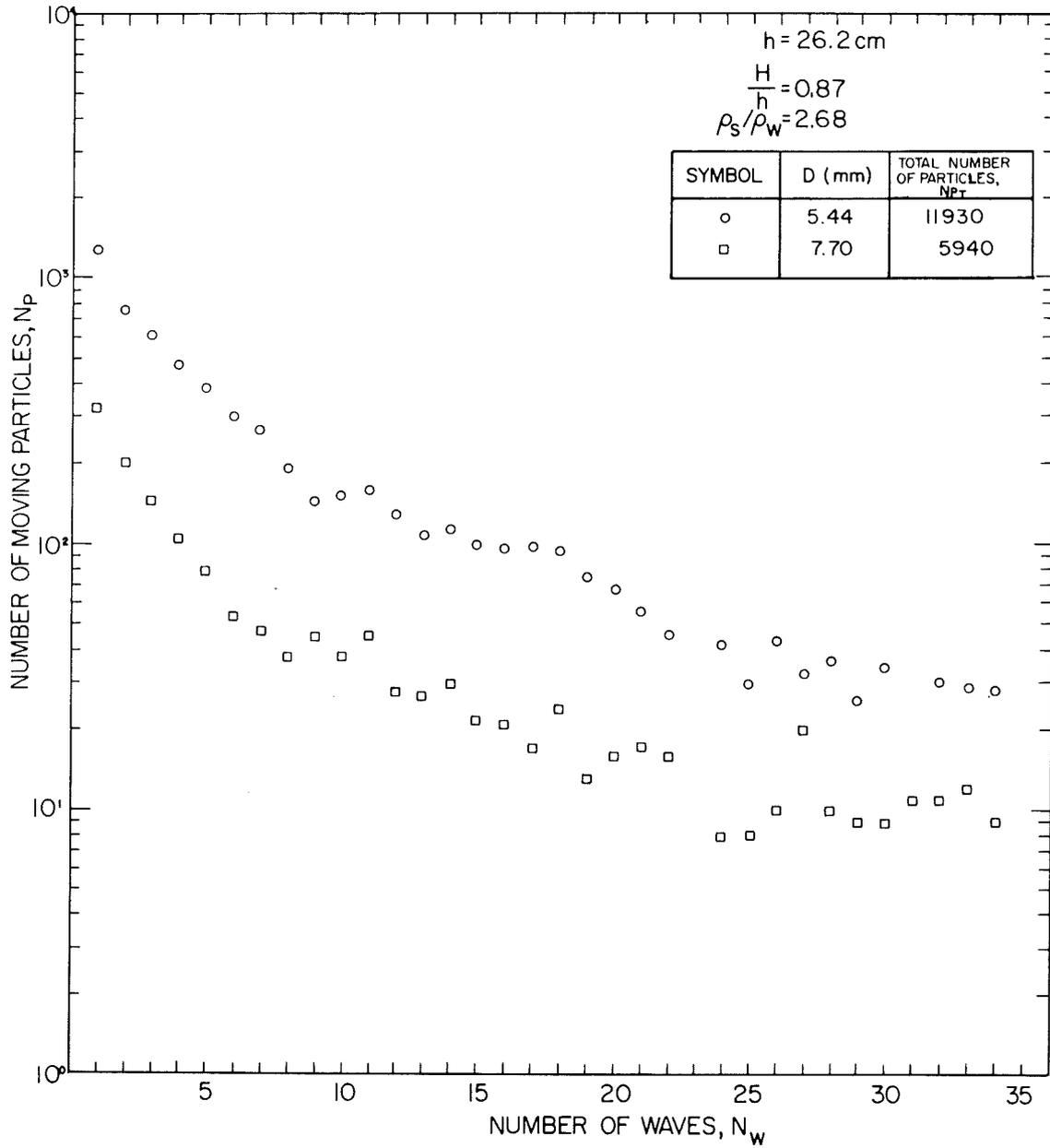
Fig. 5.15 The packing of a granular bed by waves.
