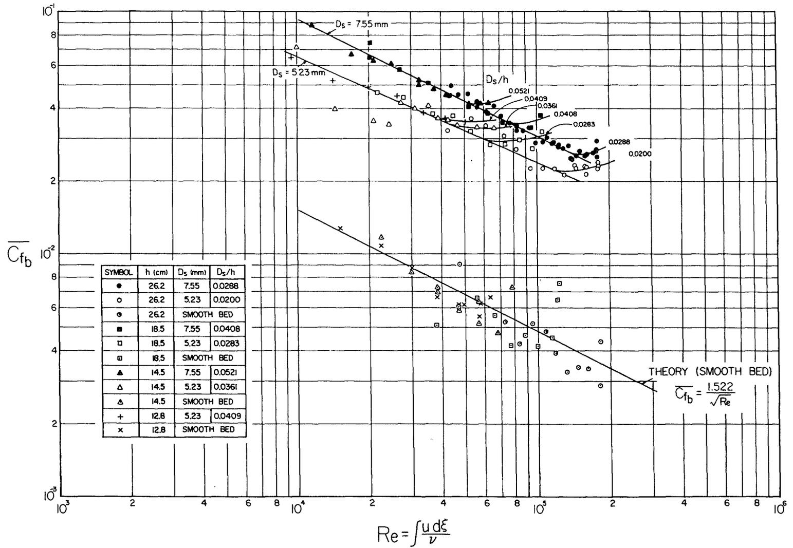
Fig. 5.11 The mean resistance coefficient as a function of the flow Reynolds number.
