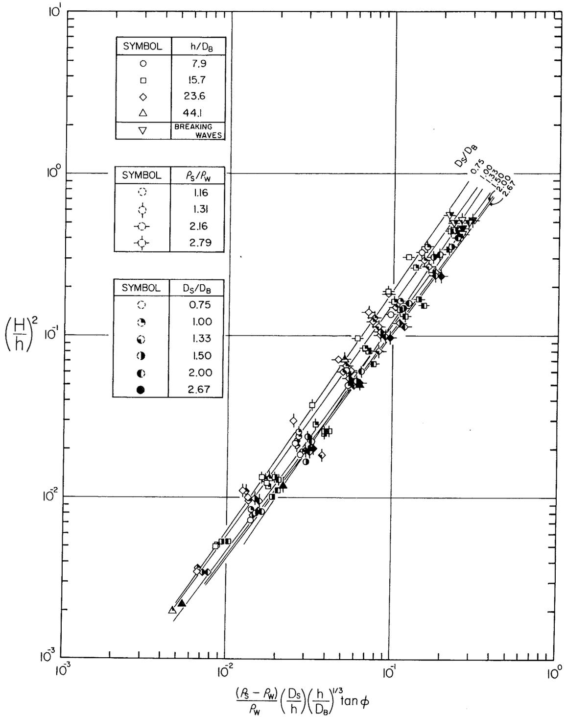
Fig. 5.26 Incipient motion of a sphere. Relationship between the wave height, the water depth, the test sphere diameter, the bed sphere diameter, the angle  $\phi$ , and the submerged density of the sphere.
