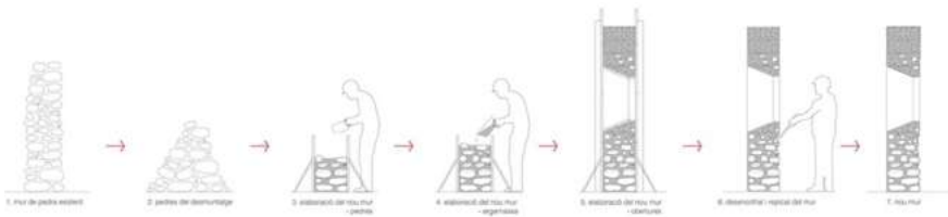
Figure 142 Wall Construction Process Casa 1413 ( https://www.harquitectes.com/wp-content/uploads/2023/03/1413-harquitectes-casa-ullastret-35.jpg )
