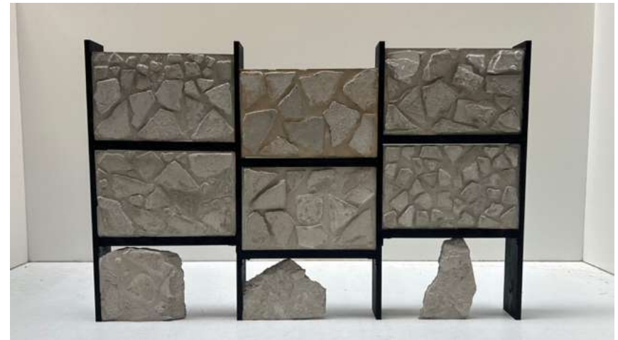
Figure 172 Demonstrator Shelf With Cracked Experiment Samples (Bottom)
