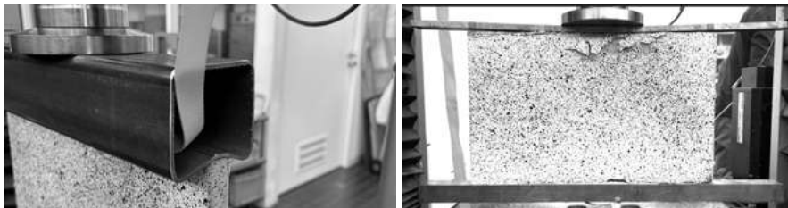
Figure 81 S2 Load Test: Bent Steel Profile (left) Point Load (right)
