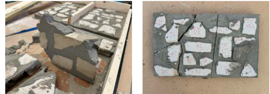
Figure 72 Breakage During Handling
