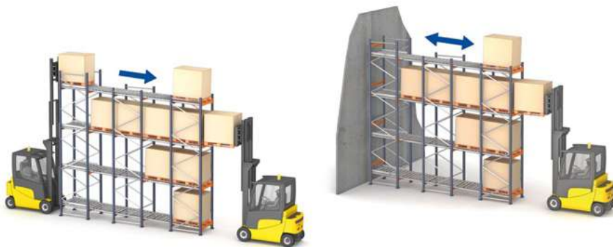
Figure 180 First In First Out (FIFO) vs Last In First Out (LIFO)
