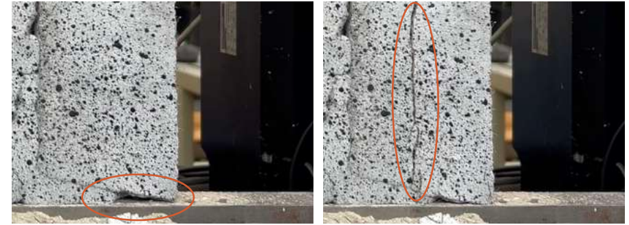
Figure 128 Zoom In W20: 1mm distance between wall and ground (left), crack through rubble
