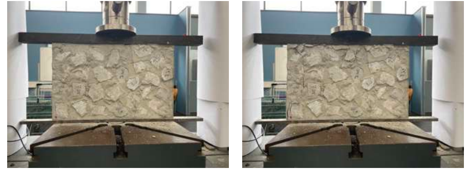
Figure 67 Wall 8 Before And After Compressive Failure
