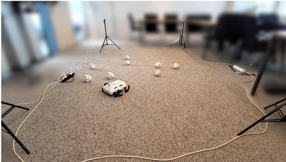
Figure 8.1: Physical validation setup during a representative run of scenario C, corresponding to the scenario definitions in Table 8.2. The obstacle stands are placed in the central part of the workspace, forcing the rover to navigate through the cluttered region before reaching the goal-side part of the test area.
