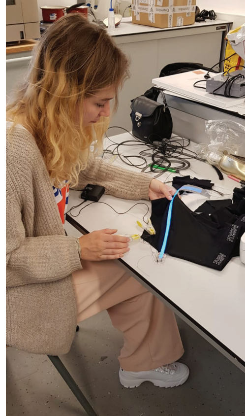
figure 74: Testing the EL strips, they still work after being sewed in.
