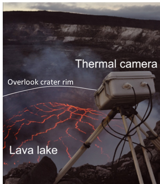
Figure 17: Thermal camera positioned at the edge of the Halema'uma'u crater observing the lava lake. The edge of the Overlook crater, the crater which houses the lava lake within the Halema'uma'u crater is highlighted for clarity. Edited from Poland and Carbone [2016].
