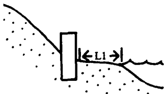
SHORE PROFILE AFTER SHORELINE RETREAT WITH SEAWALL
