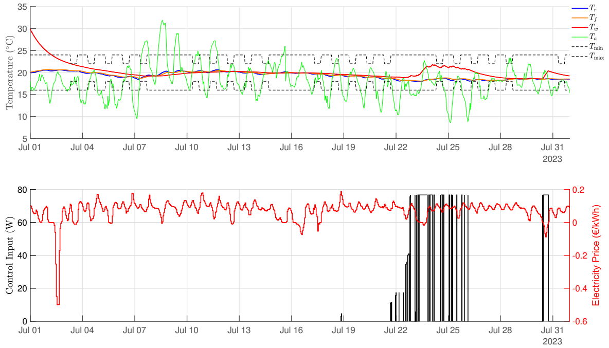
Figure 4-8: Simulation results for MPC-V during July 2023 with N_{\text{ext}} = 48 .
