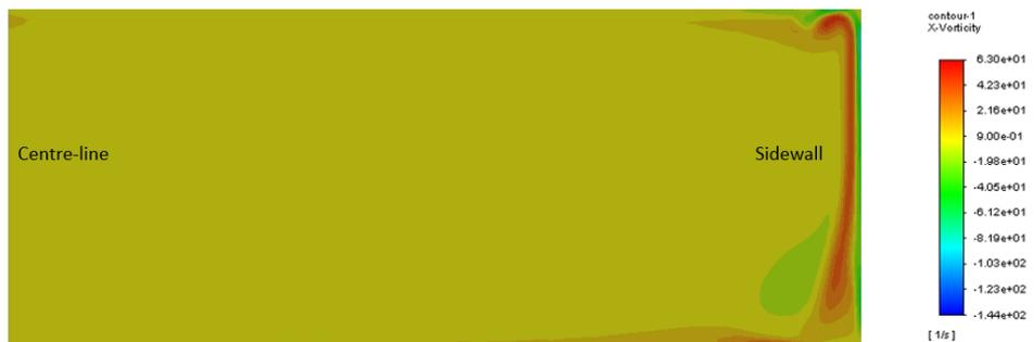
Figure 4.33: Unsteady Solution: X- Vorticity without Perturbations at Contraction Outlet  $x=0.175$
