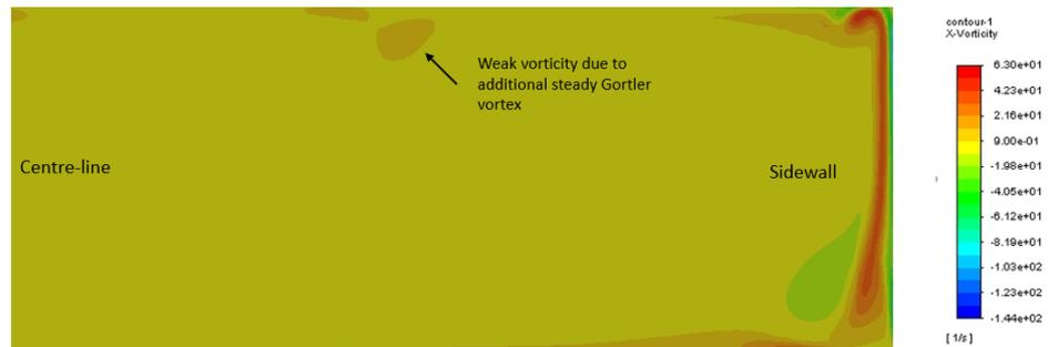
Figure 4.34: Unsteady Solution: X- Vorticity with additional Gortler Vortices at Contraction Outlet  $x=0.175$
