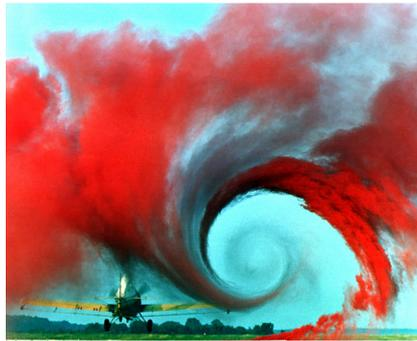
Figure 1.14: Wing-tip vortex due to aircraft wing
