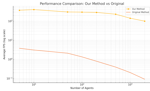
Figure 16: Comparison of FPS vs. number of agents (logarithmic scale) between the original CPU-based method and our GPU-based method.
