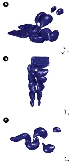
**Figure 2.10** – Vortex topology for the rolling wing case ( $t = 5.0$ ). Flapping parameters:  $St = 0.25$ ,  $froll = 1.0$ ,  $Re = 500$ . A) Perspective view, B) Top view, In this view right wing-tip corresponds to the hinged extreme. C) Side view. Adapted from Guerrero [25]
