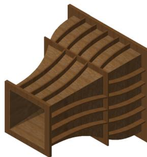
Figure 6.5 – Layout of the contraction nozzle.
