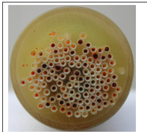
Fig. 12 Concentrate side after 40 runs (after hydraulic cleaning)
