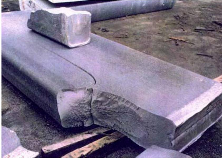
**Fig. 4.1** A photograph showing a high-strength aluminum alloy slab failed spontaneously after casting through cold cracking. The 500 kg part broke apart and was projected several meters away [1].
