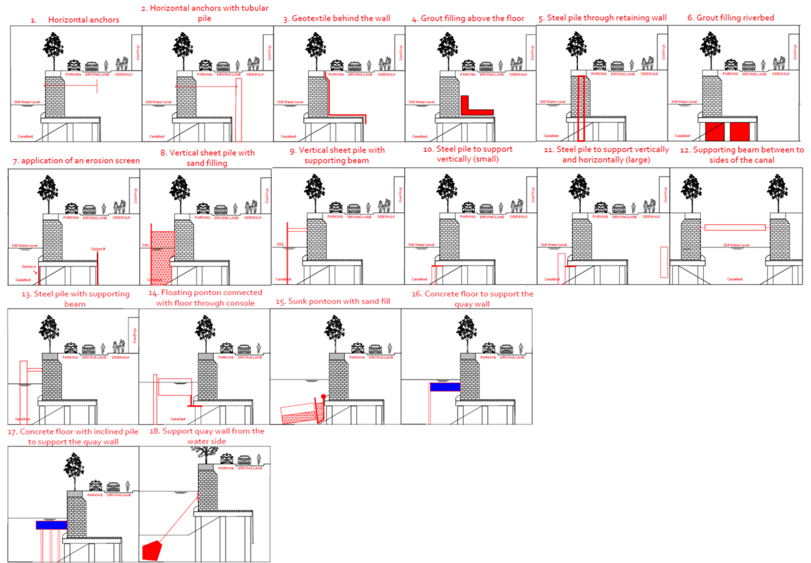
Figure 10 Intervention measures increasing the resisting forces (>R) (own illustration)
