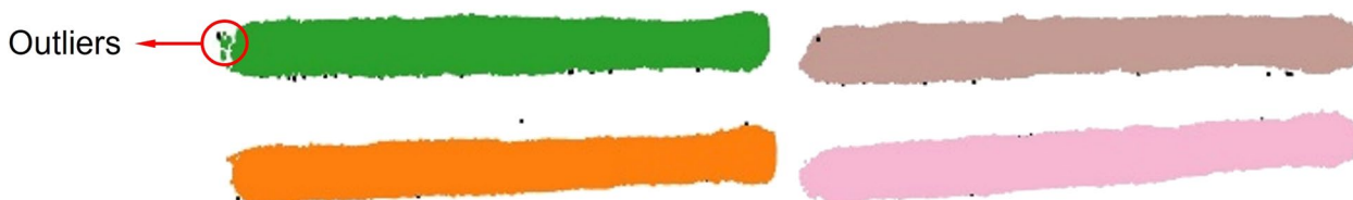
Fig. 5 Segmentation of a point cloud into multiple objects, each colour represents an object and/or outliers
