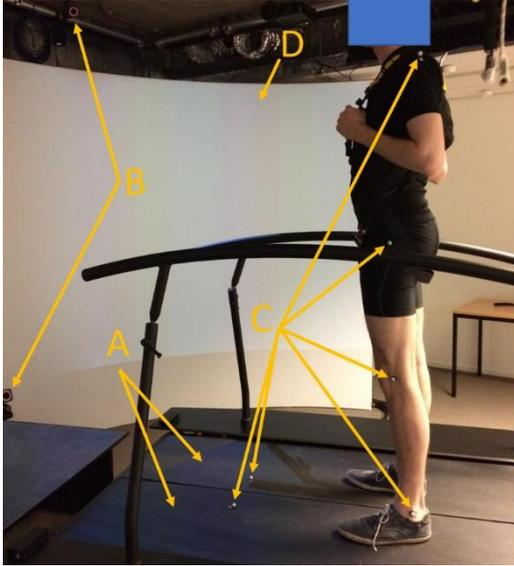
Figure 2: GRAIL system with dual belt instrumented treadmill (A), motion capture cameras (B), subject, motion capture markers (C) and semi-cylindrical screen (D).
