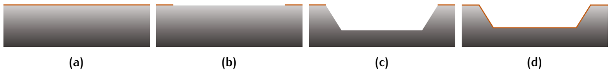
Figure 4.4: Process flow: Preparation of the substrate. (a) 200 nm LPCVD Nitride deposition as hard mask; (b) Nitride RIE etching of cavity pattern; (c) KOH etching of the well on silicon substrate; (d) 500 nm LPCVD nitride deposition for insulation.
