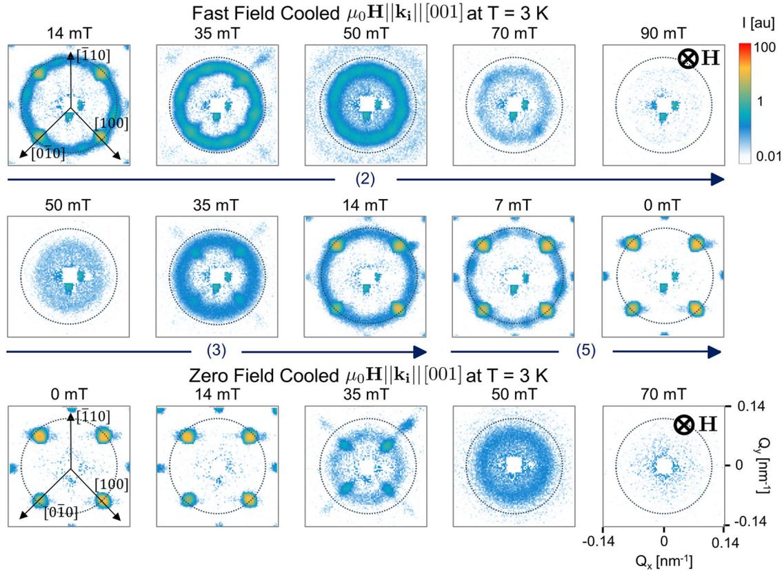
**Fig. 4** SANS patterns recorded at  $T = 3$  K and with the magnetic field applied along the [001] crystallographic direction. The magnetic field was applied parallel to the incoming neutron beam ( $\mathbf{H} \parallel \mathbf{k}_i$ ) following the fast field cooled (FFC) and zero field cooled protocols. The arrows and numbers below the SANS patterns indicate the step of the FFC protocol, as defined in Fig. 1, for which the measurements were performed
