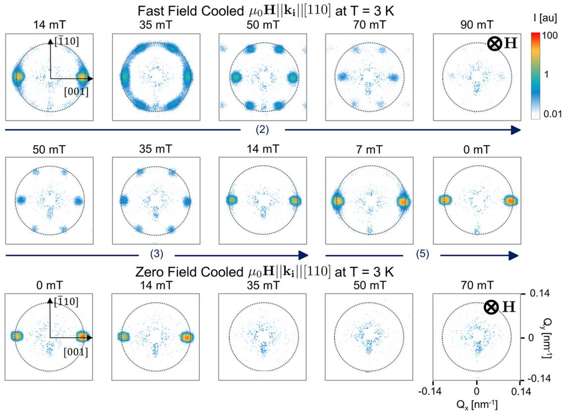
**Fig. 3** SANS patterns recorded at  $T = 3$  K and with the magnetic field applied along the  $[110]$  crystallographic direction. The magnetic field was applied parallel to the incoming neutron beam ( $\mathbf{H} \parallel \mathbf{k}_i$ ) following the fast field cooled (FFC) and zero field cooled protocols. The arrows and numbers below the SANS patterns indicate the step of the FFC protocol, as defined in Fig. 1, for which the measurements were performed
