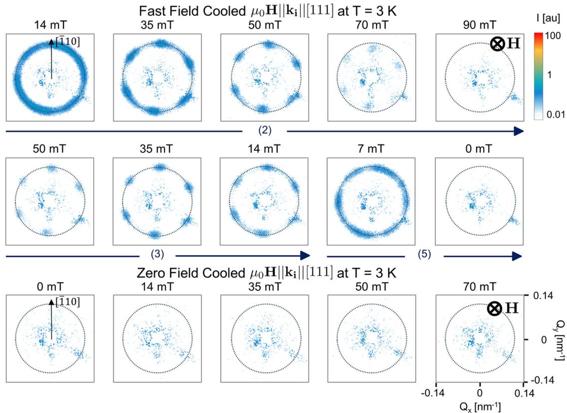
**Fig. 2** SANS patterns recorded at  $T = 3$  K and with the magnetic field applied along the [111] crystallographic direction. The magnetic field was applied parallel to the incoming neutron beam ( $\mathbf{H} \parallel \mathbf{k}_i$ ) following the fast field cooled (FFC) and zero field cooled protocols. The arrows and numbers below the SANS patterns indicate the step of the FFC protocol, as defined in Fig. 1, for which the measurements were performed
