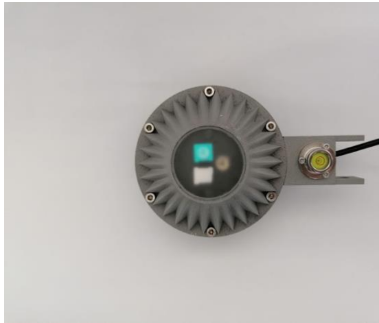
Figure 14: Grey albedometer with N-BK7 Ground Glass Diffuser
