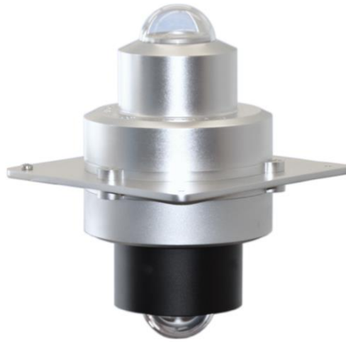
Figure 8: Spectrafy SolarSIM Albedometer consisting of two SolarSIM-G spectral irradiance sensors [10].
