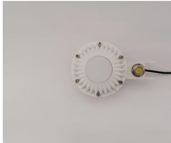
Figure 15: White albedometer with Hybrid diffuser
