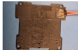
Figure 4. PCB with LabIR paint of known emissivity ( \epsilon_{IR} = 0.8 ) for Test 2
