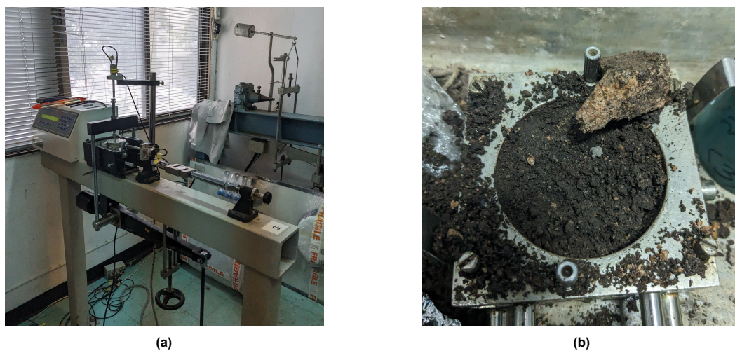
Figure 4.4: Direct shear test in the laboratory (a) using remolded samples due to stones in the undisturbed samples (b).
