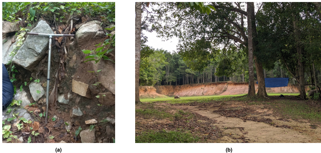
Figure 4.3: Soil depth estimation in the field (a) using a manual hand auger and (b) visible soil profiles in the field.
