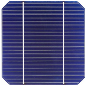
Fig. 7: Example of a monocrystalline silicone cell Homogenous structure (Direct Industries, n.d.)
