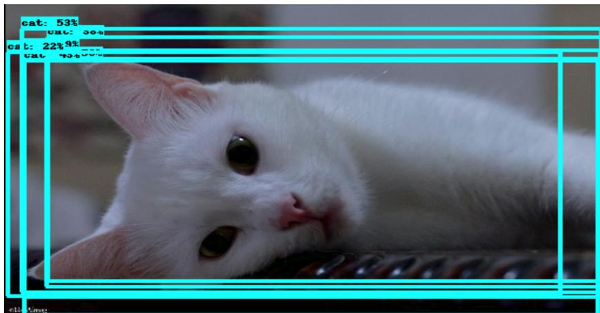
**Figure 5.2:** Multiple detected boxes appear given the object fits multiple differently shaped bounding boxes, each having a different confidence score, from [82].
