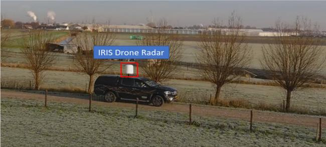
Fig. 4. IRIS radar by Robin Radar Systems B.V. anchored on the moving vehicle.
