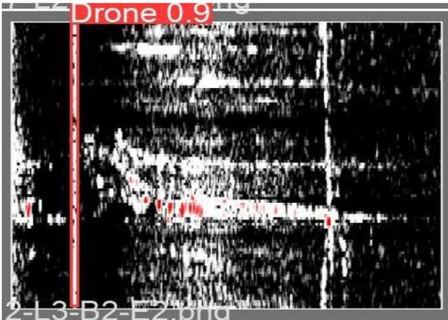
Fig. 6. Example of output of the proposed model for the same range-Doppler plot of Fig. 5, but using Adam as optimizer. The choice of this optimizer did not yield false detections.
