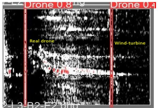
Fig. 5. Example of output of the proposed model, with detections obtained using SGD optimizer. A false alarm induced by the a wind turbine is reported, near a true detection.
