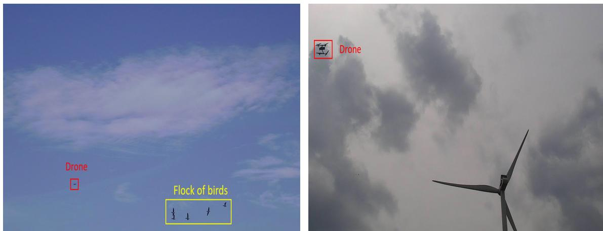
**(a)** Faraway drone that is seen as a single point, with a flock of birds flying in front of the camera.
