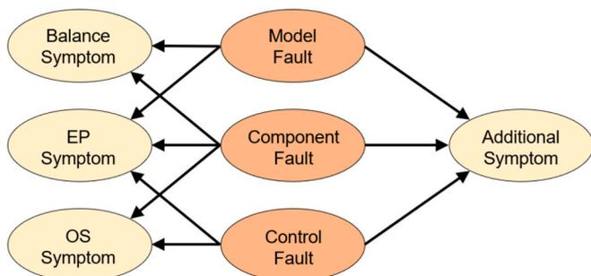
Fig. 4. Illustration of the general 4S3F BN structure [11,17,46,71].
