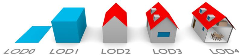
Figure 1.2: Levels of detail [Biljecki et al., 2016]
