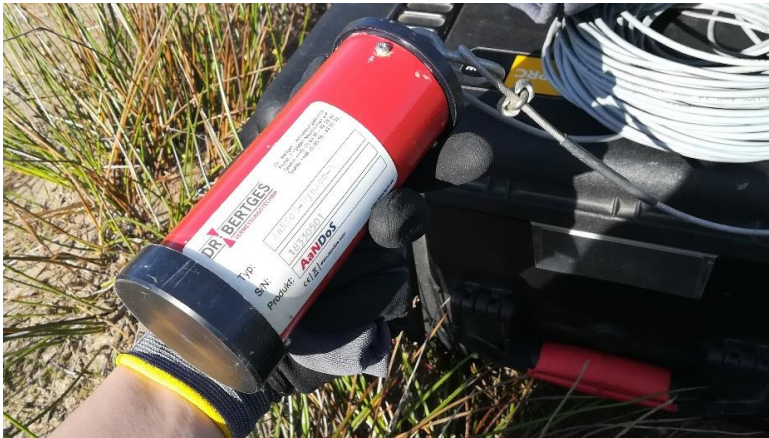
Figure 6.3: Aluminium cylindrical casing containing the pore pressure transducers assembled by Dr. Bertges.
