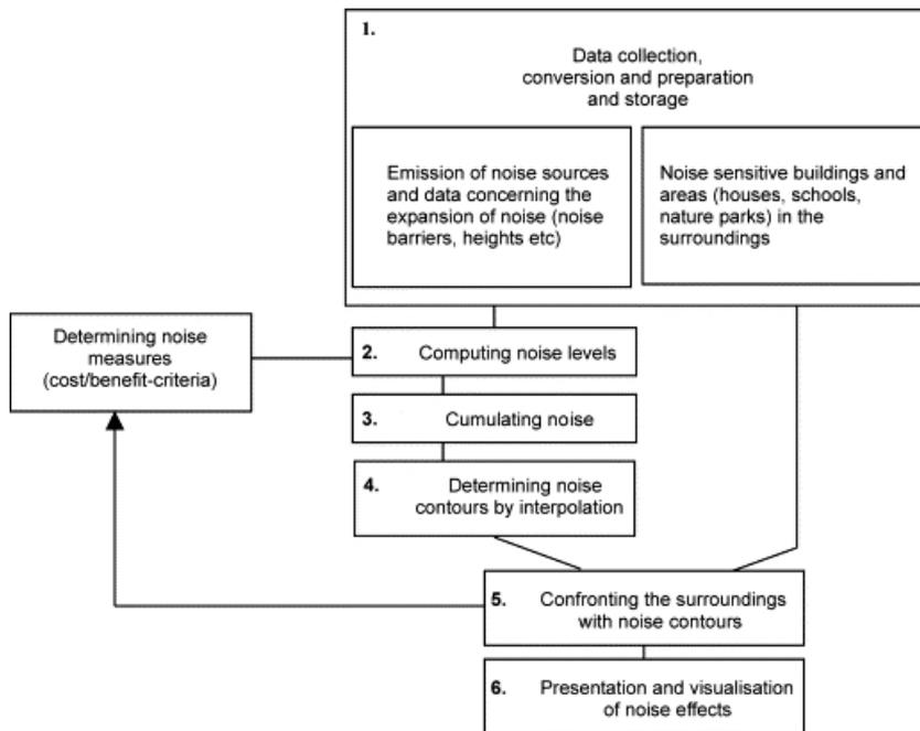
Figure 2: Schematization of the noise mapping process (de Kluijver and Stoter, 2003).
