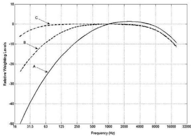
Figure 1: Approximate electrical frequency response of the A-, B-, and C-weighted networks of sound level meters (Munjaj, 2013).
