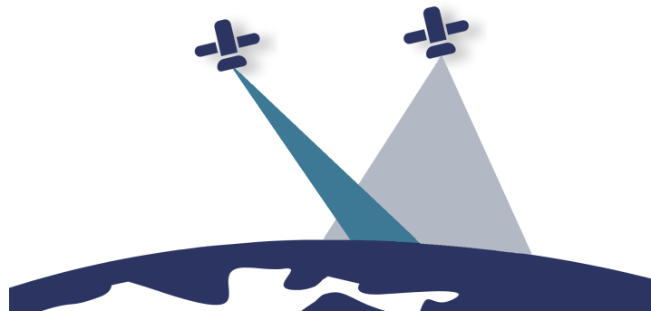
Figure 2.1: Conceptual illustration of the AI-based Tip and Cue formation. The leading Tip satellite scans a wide area with a large field-of-view sensor, while the following Cue satellite performs off-nadir pointing to acquire high-resolution imagery of a detected target.
