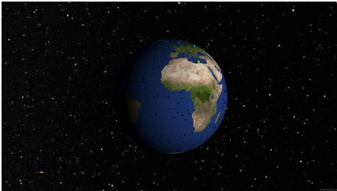
Figure 6.50: Orbital simulation snapshot showing the global distribution of targets (blue), detection outcomes (true positives in green and false negatives in red), and satellite positions during the simulation. The interactive PyVista visualization is updated in real time, while in automated workflows it is hidden and outputs are recorded.
