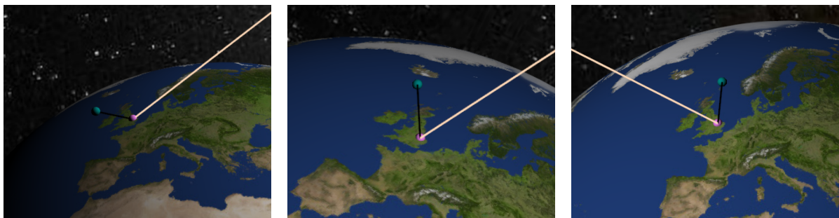
Figure 6.34: Geometric verification of maximum glint positioning at three different times of day. For each configuration, the satellite, in blue, is placed along the specular reflection direction of the incident solar ray with respect to the local surface normal, satisfying the mirror-reflection condition.
