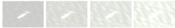
Fig. 16. Simulated off-nadir renderings of the same target at varying solar incidence angles. Cue satellite and target positions are held constant, isolating the effect of illumination geometry. Satellite image © 2022 Maxar Technologies.
