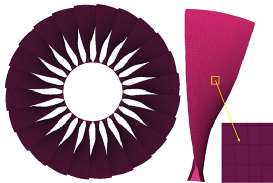
Figure 3. Finite element model of turbofan engine fan.
