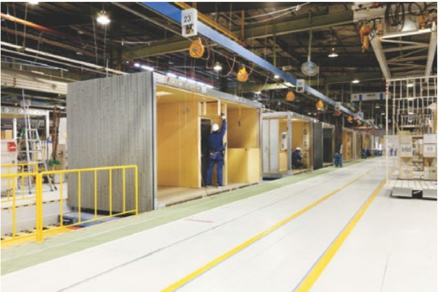
Figure 5.5. Linear production in Sekisui Heim factory (Bock, T, Linner, T, Robotic Industrialization , 2015)
