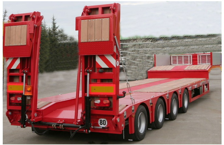
Figure 5.20. Low loader platforms. ( toptrucks.nl , 2017)
