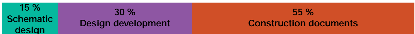
Figure 4.24. Distribution of design stages in design phase in traditional construction (source: Prefab Architecture, Timberlake, J., 2010 )
