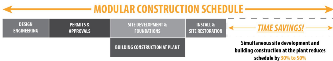
Figure 7.4. Comparison of on-site and modular construction process (Modular Building Institute, 2016)
