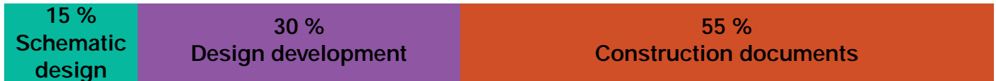
Figure 4.22. Distribution of design stages in design phase in traditional construction (source: Prefab Architecture, Timberlake, J., 2010 )
