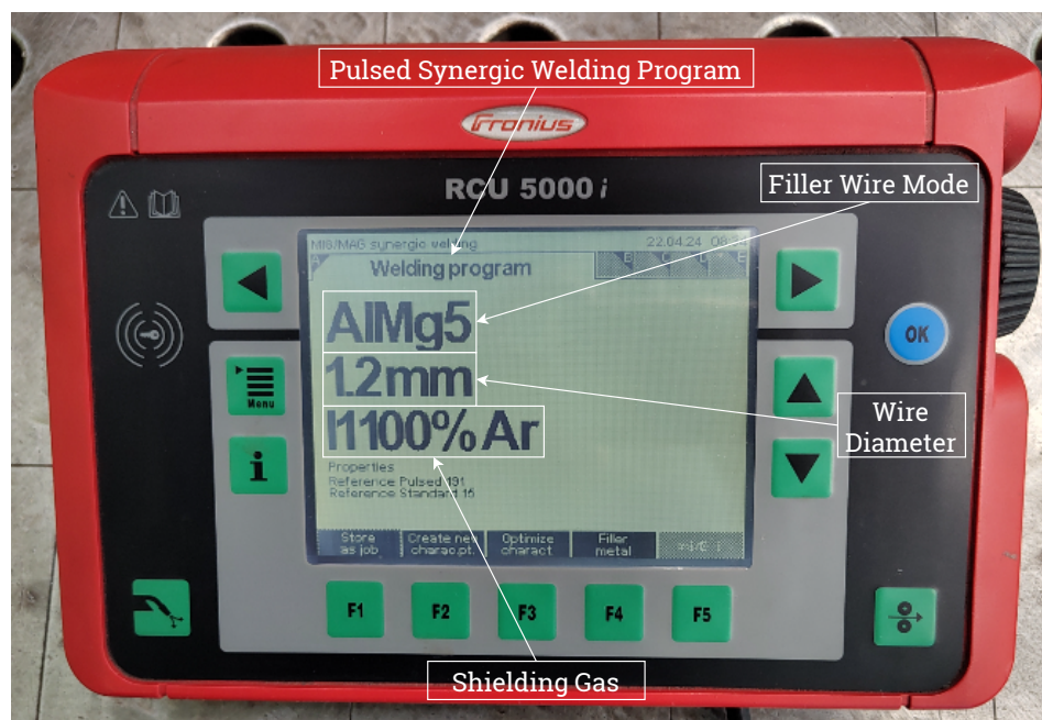
Figure B.3: Pulsed Synergic Welding Program in TransPuls Synergic 3200 CMT R and TransPuls Synergic 5000 R welding source machines by Fronius International GmbH
