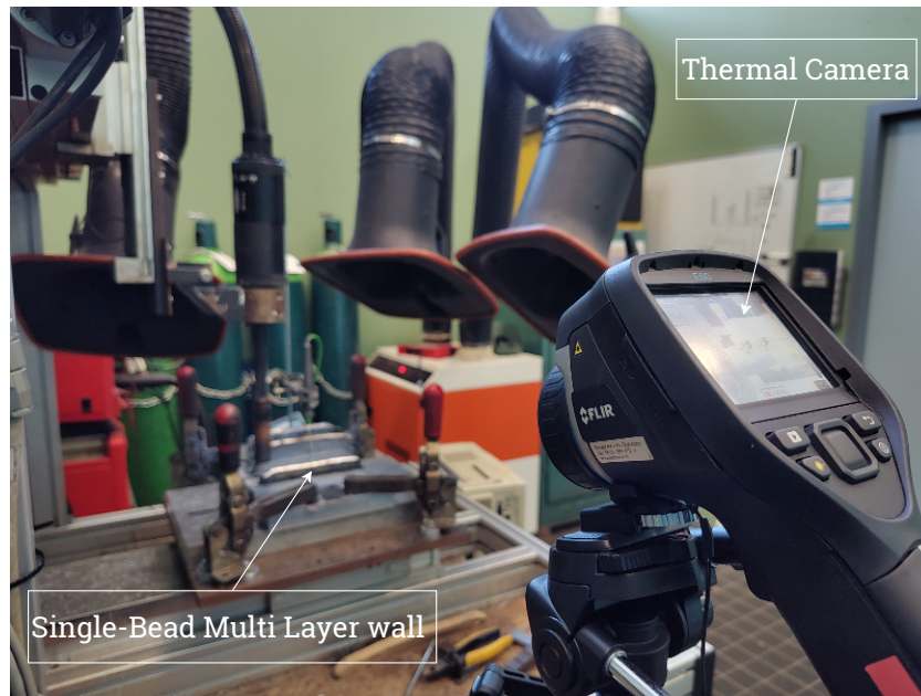
Figure 3.8: Inter-layer temperature measurements using thermal camera
