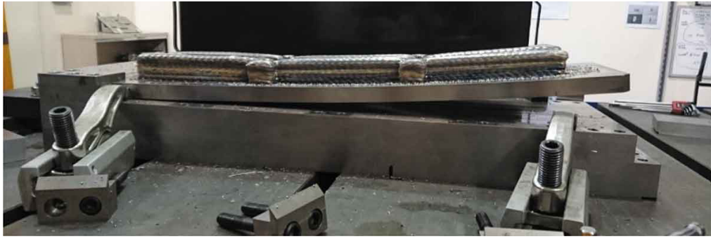
Figure 1.2: Distortion in component fabricated using WAAM [15]
