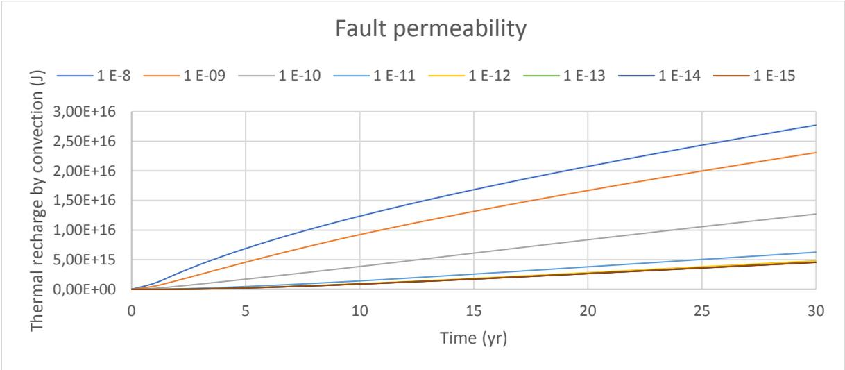
Figure 18 Thermal recharge with varying fault permeability
