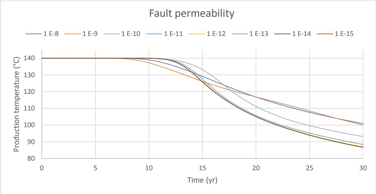
Figure 19 Production temperature with varying fault permeability
