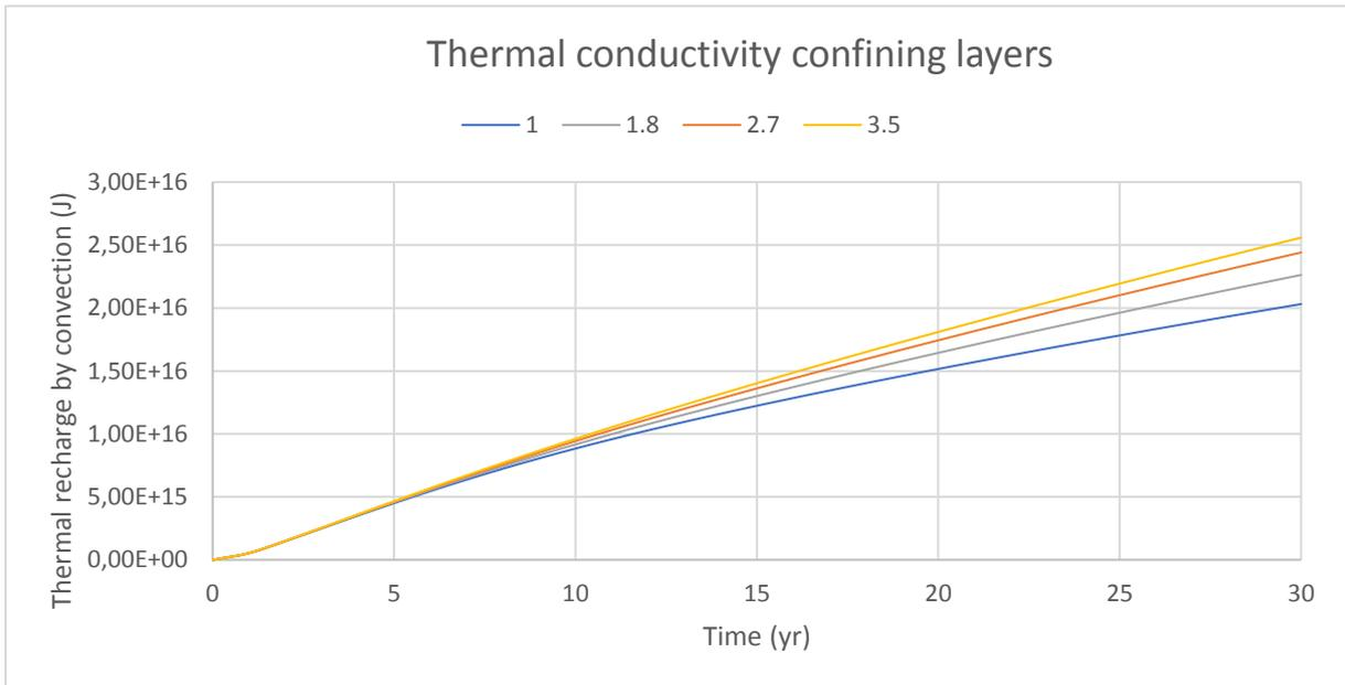
Figure 22 Thermal recharge by convection with varying thermal conductivity of confining layers
