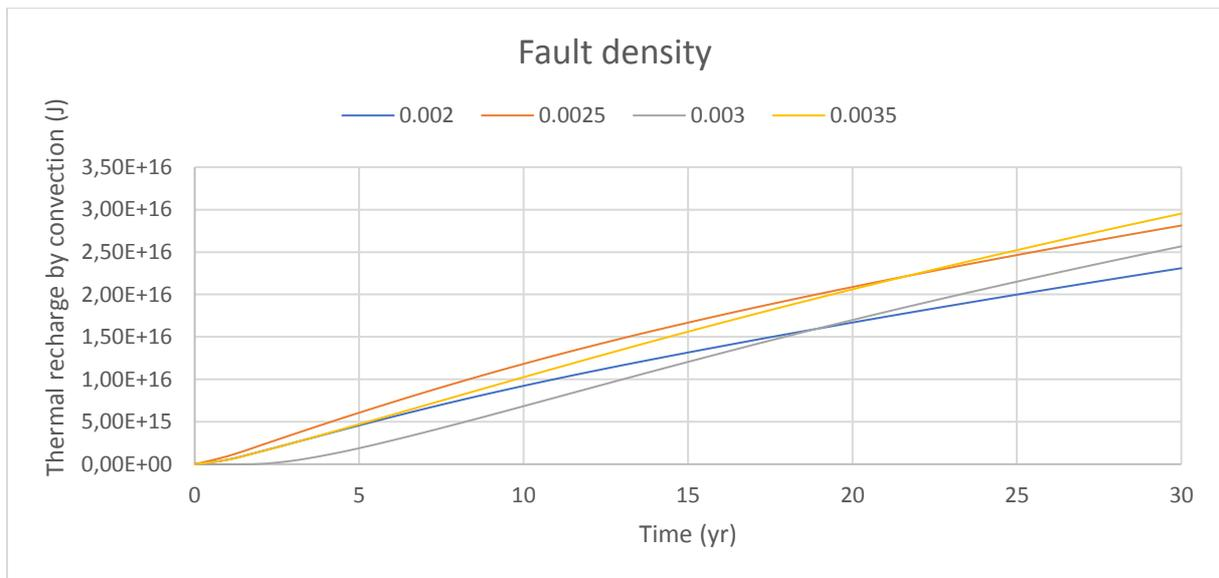
Figure 16 Thermal recharge by convection with varying fault density
