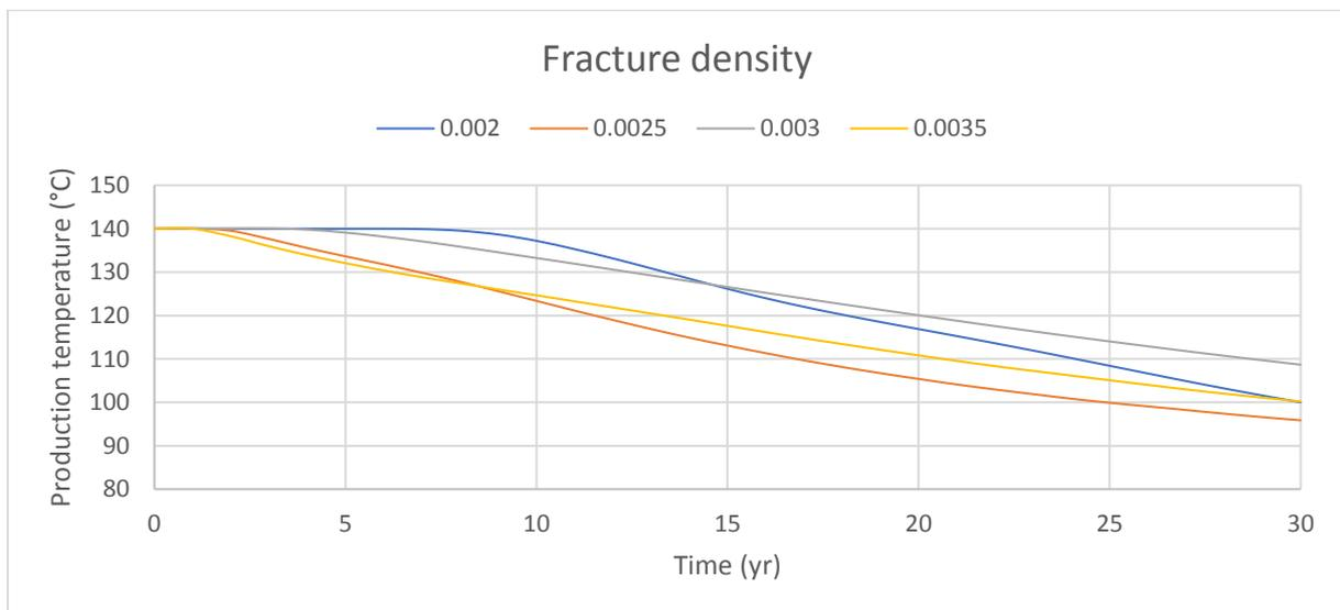
Figure 17 Production temperature with varying fault density
