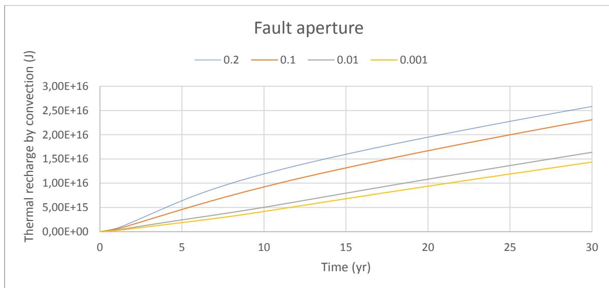
Figure 12 Thermal recharge by convection with varying fault aperture
