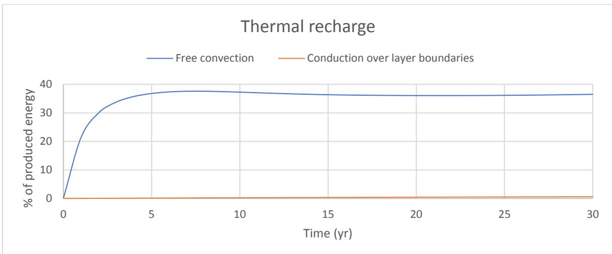
Figure 12 Free convection and conduction as a percentage of production energy
