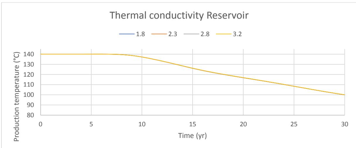
Figure 11 Production temperature with varying thermal conductivity of reservoir rock
