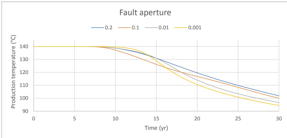
Figure 13 Production temperature with varying fault aperture
