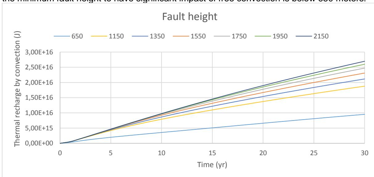
Figure 14 Thermal recharge by convection with varying fault height
