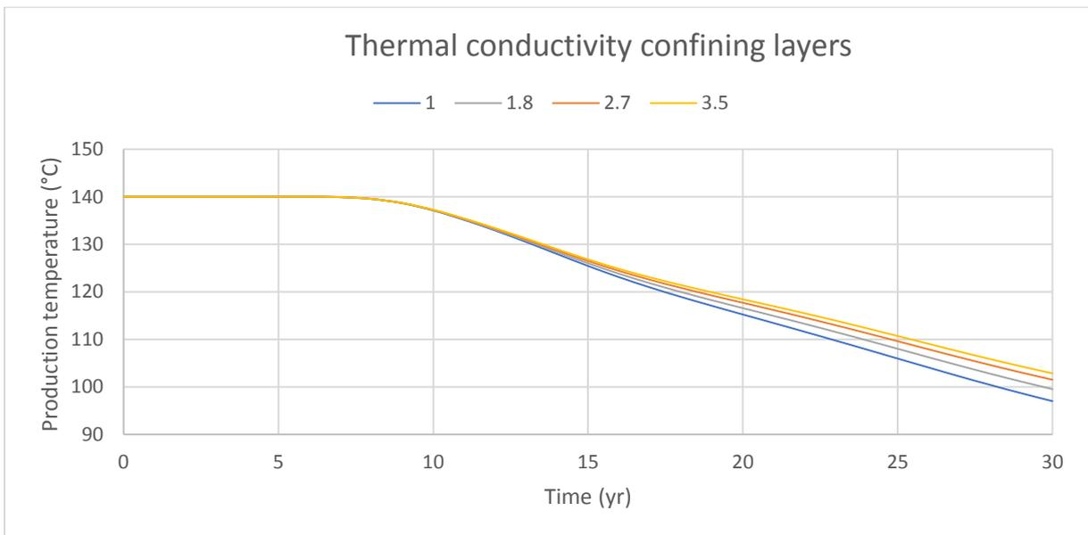
Figure 23 Production temperature with varying thermal conductivity of confining layers
