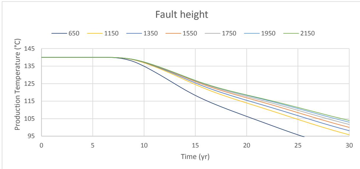
Figure 15 Production temperature with varying fault height
