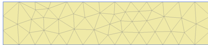
Figure 66: Mesh Geonor sample
