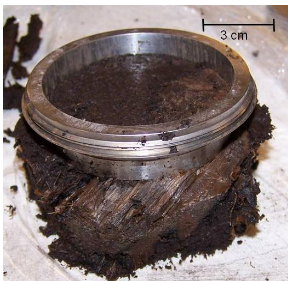
Figure 26: Sample a15 surmounted by the hand cutting ring
