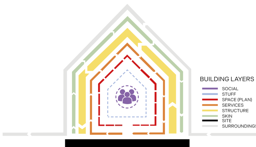
Figure 3-3 Building layers model. Adapted from Schmidt III and Austin (2016)
