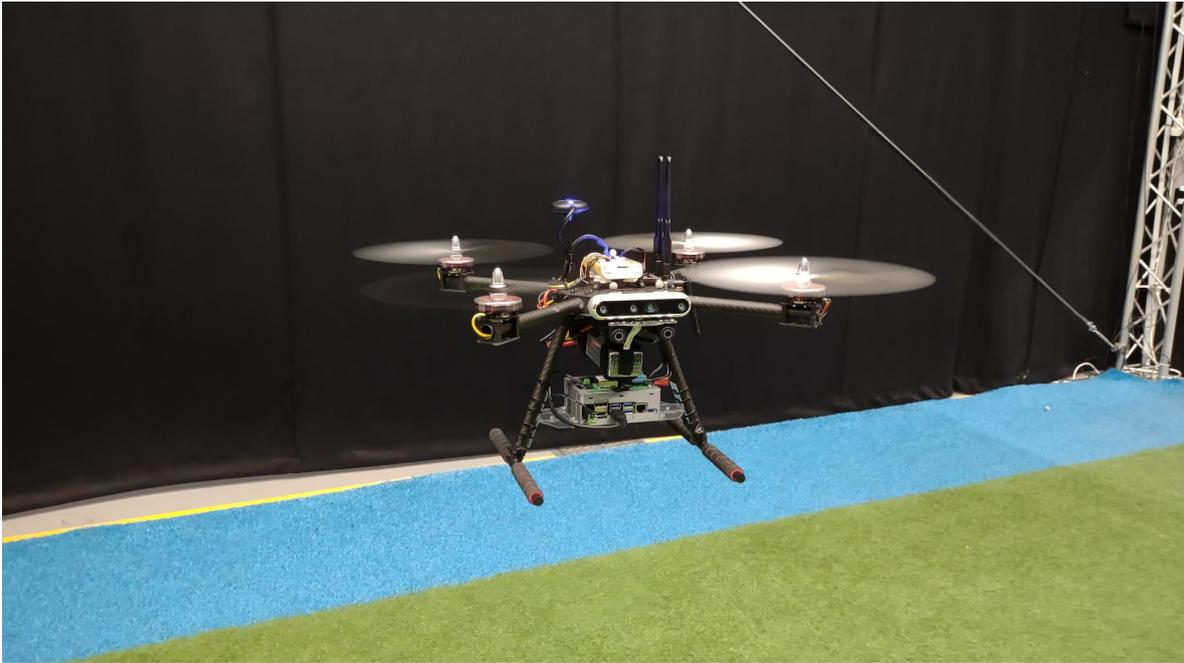
**Figure 3-3:** HoverGames quadrotor flying in the lab environment.
