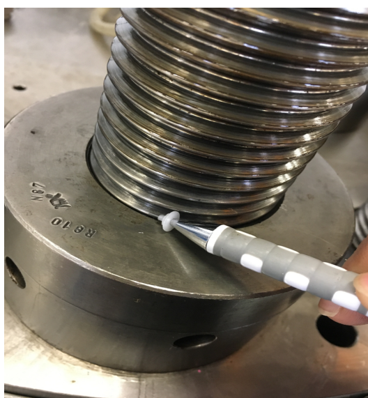
Figure 4-6: Simulated crack at bolt thread using Hsu-Nielsen source.
