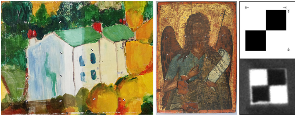
Fig. 3. Evaluation artifacts. Left: color image of the mock-up painting, with landmarks. Middle: color image of the Byzantine icon, with landmarks. Right: the design used to print landmarks (top) and close-up on an imaged landmark (bottom).
