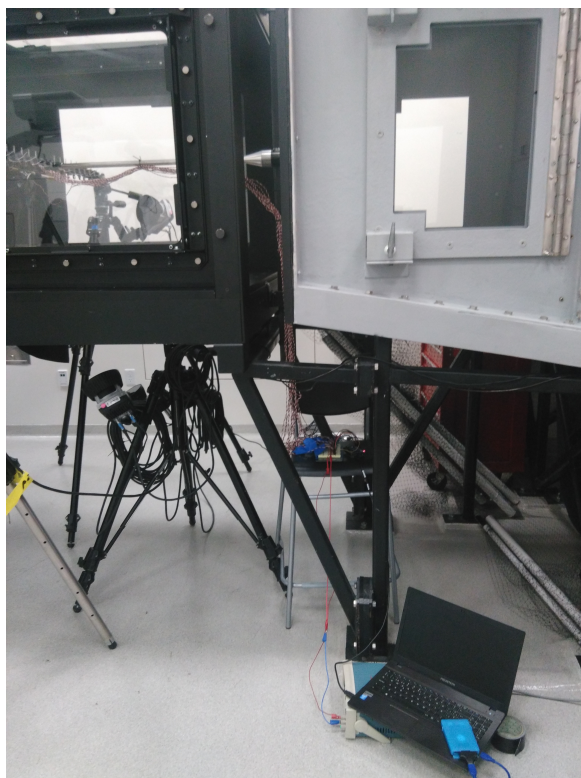
Figure A.5: Array wiring to Arduino board and XBee module.
