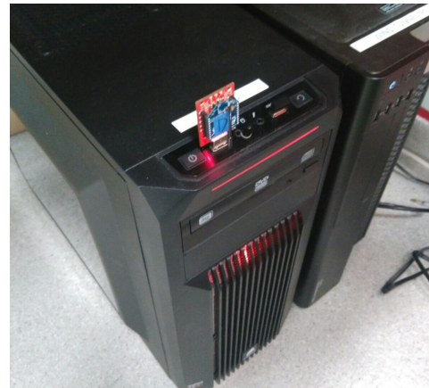
Figure 3.16: XBee module connected through a USB Dongle to PC. Wind sensors measurements are transmitted wirelessly to the PC with Labview.
