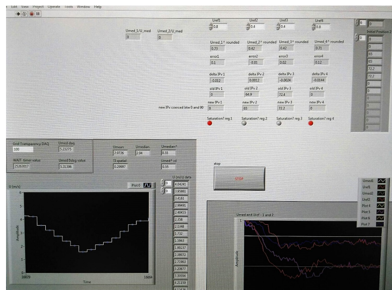
Figure A.7: Labview VI user screen for 4-region closed-loop controller designing wake gust.
