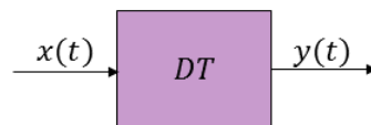
Figure D.1: Block diagram for dead time element. Input and output time signals, x(t) and y(t) are shown
