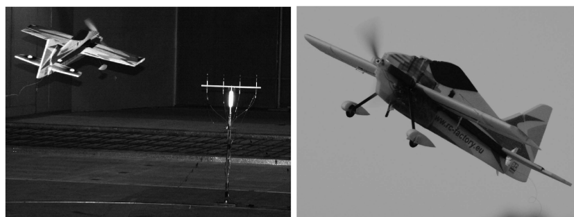
Figure 1.4: Testing of fixed-wing unmanned aerial vehicle in wind tunnel and in open-air flight. From the work by Abdulrahim et al. (2010). Picture on the left shows the fixed-wing UAV and the Cobra probes mounted in the wind-tunnel test section for flow measurement.
