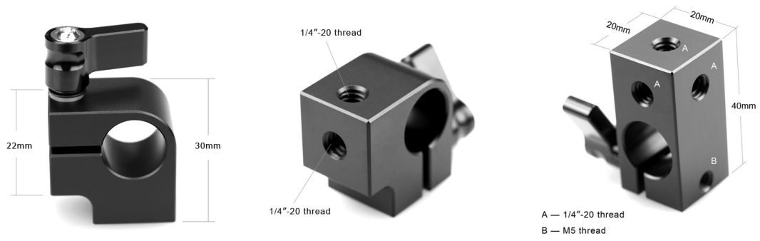
Figure A.8: Types of clamps used for the array setup. Left and center show the clamps used to hold sensors (wind sensors and hotwire probe); right shows the rectangular clamp used to attach the array to the wind tunnel traverse. Images from SmallRig (2017) .
