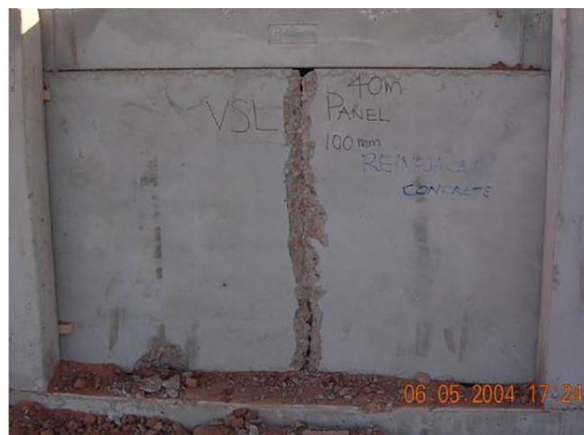
Figure 2.1: Panel 4 after the blast
