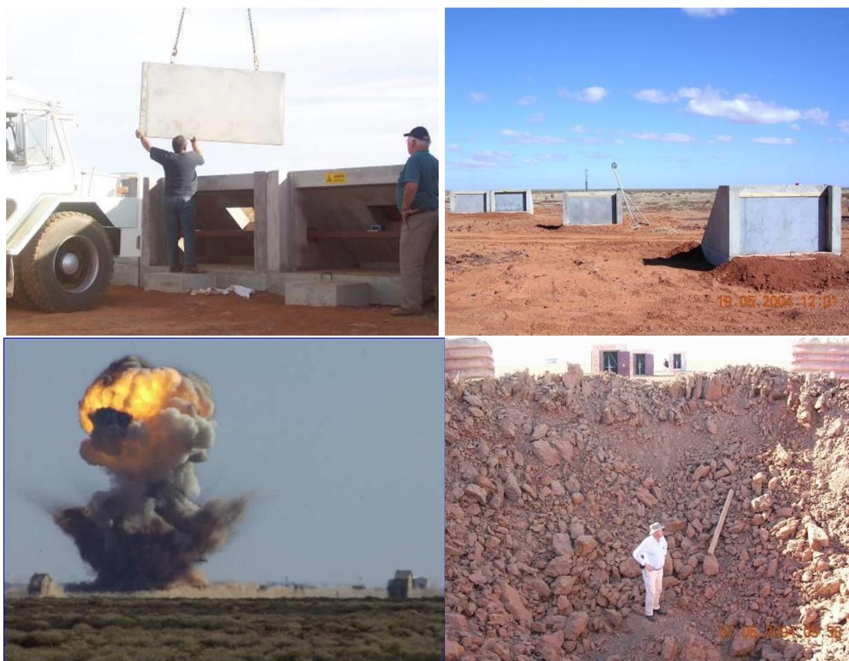
Figure 1.1: Installing panels into concrete frames (top left), Panels ready for blast (top right), Blast, equivalent to 6t of TNT (bottom left), Crater (17m diameter) caused by the blast (bottom right)
