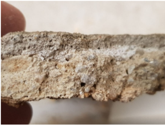
Fig. 26 Sample of the render of the East façade with a cementitious repair coat
