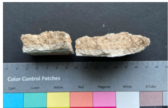
Fig. 25 Samples of the old lime render in two coats
