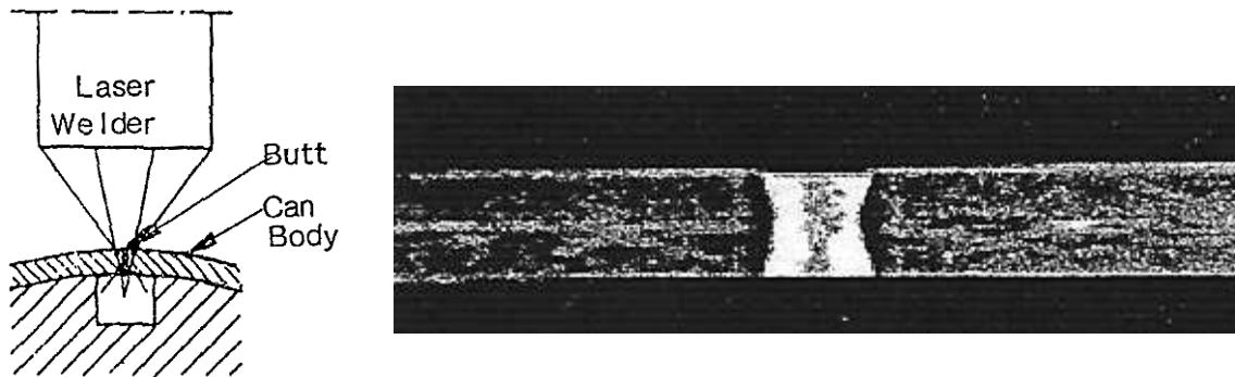
Figure 2.3: Schematic representation of the laser welding principle on the left-hand side with on the right-hand side an associated photomicrograph of a laser weld appearance [11 and 15].
