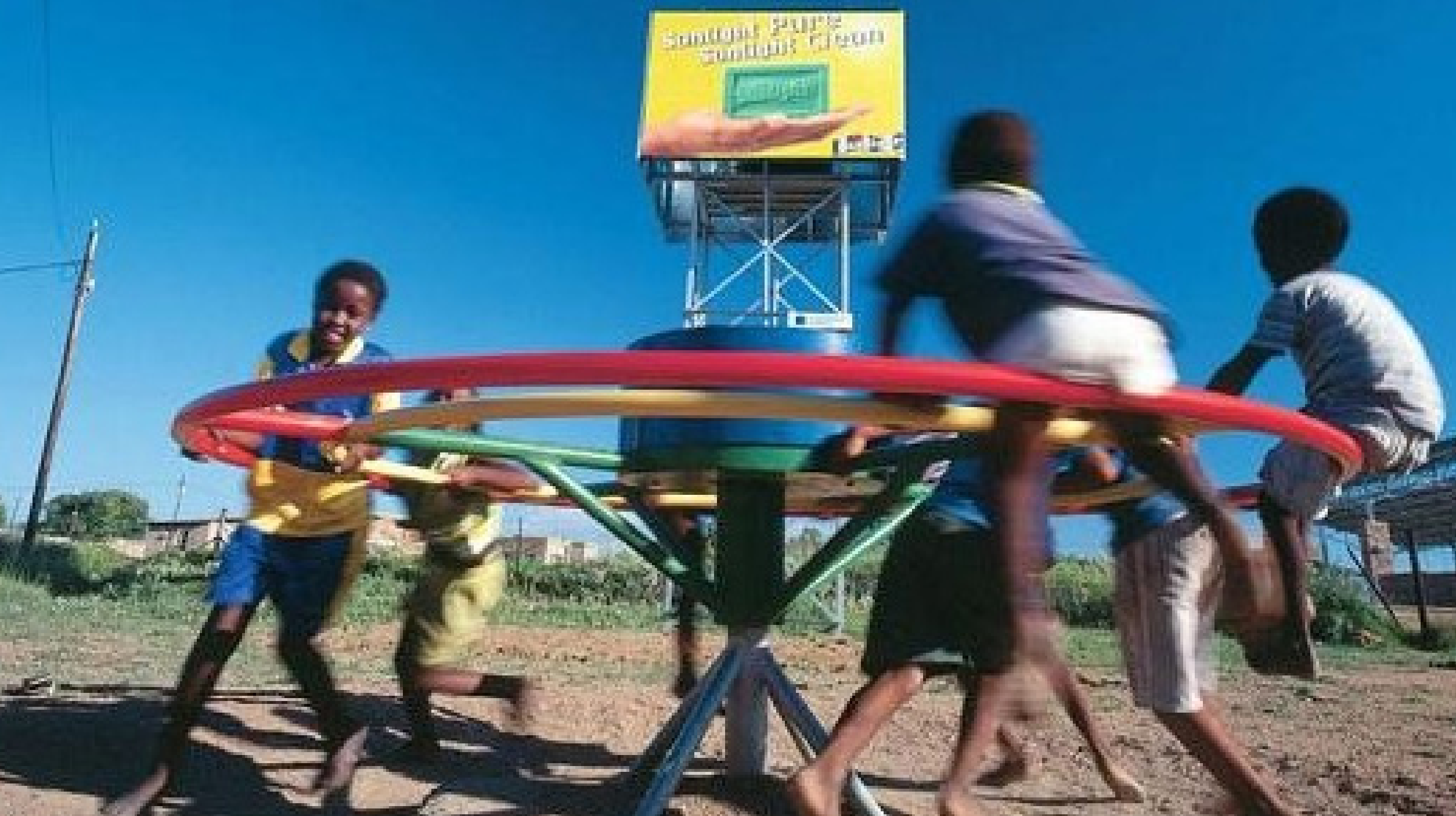
Figure 16: The intention of the playpump was children playing while at the same time pumping water (image left), however in reality women ended up using the pumps in an inefficient and non ergonomic way (image right). Images by Ralph Borland
