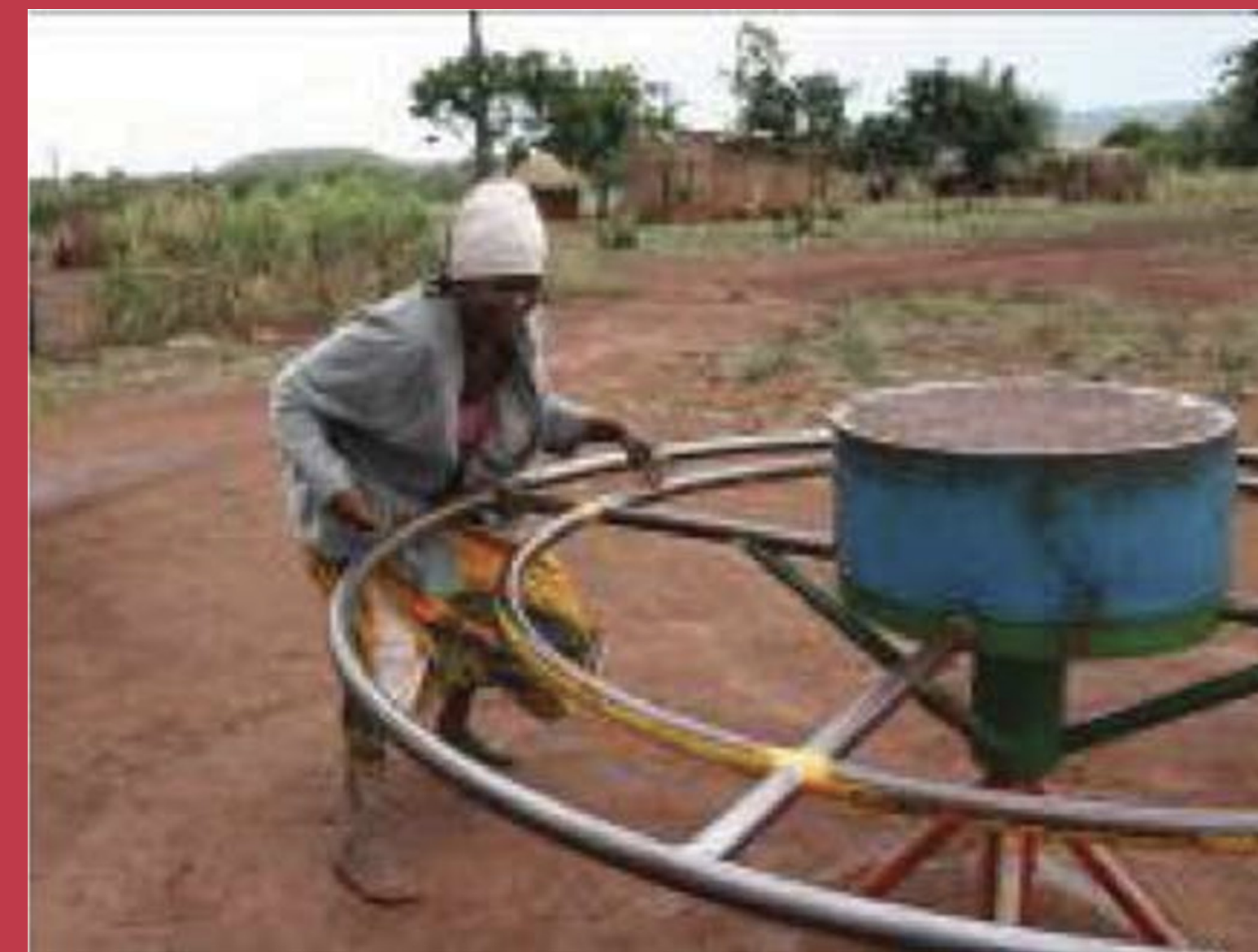
Figure 16: The intention of the playpump was children playing while at the same time pumping water (image left), however in reality women ended up using the pumps in an inefficient and non ergonomic way (image right). Images by Ralph Borland
